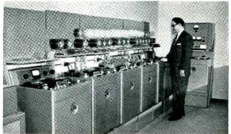
Tom Parrish runs the duplicating department. Here he examines one of the Ampex "slave" units while a batch of Pentapes is being duplicated for the Pentron Corporation. All the tape is Audiotape.
