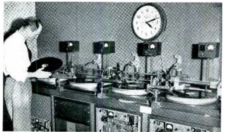
An Audiodisc is placed by Bernie Clapper on one of the four synchronized lathes in the dubbing room. This is a custom-made machine; all recording heads and turntables are driven by one motor unit in perfect synchronization.
