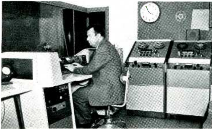
Mason Coppinger, V.P. and Chief Engineer, at work at the custom-made console in Studio B. This console allows simultaneous monaural and stereophonic recordings to be made of a performance.
