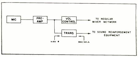
Fig. 2. Program feeds from the studio console to an external sound reinforcement mixer may be obtained by means of a bridging tansformer, or bridging pad, connected across the output of the microphone preliminary amplifier as shown. If bridging pads are used several precautions must be observed as discussed in the text.
