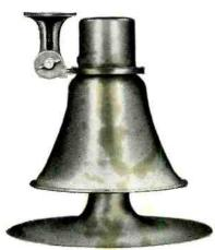
NEW RADIAL RF-ENTRANT SPEAKER, excellent for all types of industrial sound installations. Provides superlative and complete 360° speech intelligibility by efficiently over-tiding factory high noise levels. Frequency response 300-6000 cps. Handling capacity 25 watts continuous 35 w. peak. Has mounting bracket. Size 12" wide by 125%" high.
