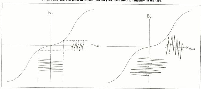
new frequency with an amplitude which is larger the greater the value of the recorded audio amplitude. This increase in amplitude is what would be expected if the demagnetization of the bias component of induction takes place according to the transfer characteristic curve for the bias frequency.
