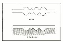
Fig. 9 Embossed track for vertical recording.
