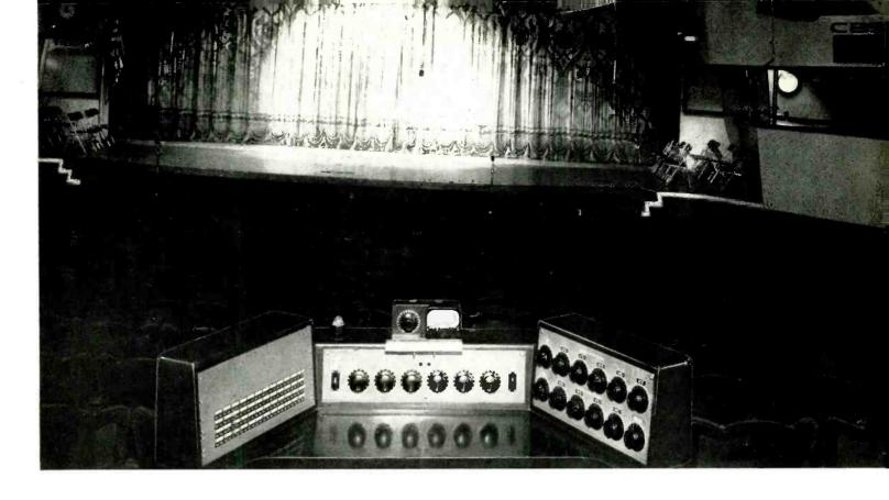
Fig. 1. A sound reinforcement control console installed in the audience area of a CBS radio theater. Such a vantage point is highly desirable for this activity as the operator has first-hand knowledge of the degree of reinforcement required and the effectiveness of all operating adjustments.
