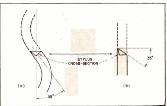
Fig. 1. The low noise-signal ratio measured in the dead groove (left) is only representative of what actually happens in one part of the a.c. alternation. Fig. 2 (right). The two methods of setting up to measure noise modulation—(a) dynamic, (b) static. At the instant shown, the stylus in (a) is just as embarrassed as the (b) stylus in its attempt to polish the sidewall to a noise-free surface.
