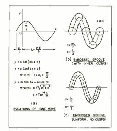
Fig. 10. In (a), method of determining minimum radius for sine curve, (b and c), embossed grooves with and without inner cusps.
