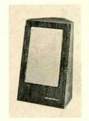
closure functions as the throat of a horn whose final extension is the walls of the room in which it is situated. High frequencies are direct-front-radiated. Total internal displacement of the unit is approximately 1½ cubic ft. Available from jobbers and dealers in hand-rubbed mahogany or blonde finish. Electro-Voice, Inc., Buchanan, Mich.
