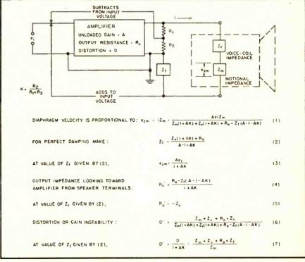
Fig. E. Combined positive and negative feedback. Formulas given here are applicable to Fig. A without change. Two other variations of the basic circuit are possible and have slightly different
