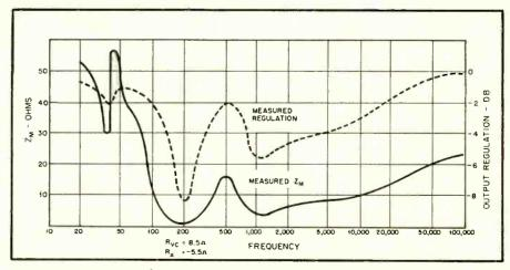
Fig. 1. Actual measured curves showing the motional impedance  $Z_{\rm m}$  for a typical speaker system (solid line) and the regulation of the driving amplifier (dotted line).
