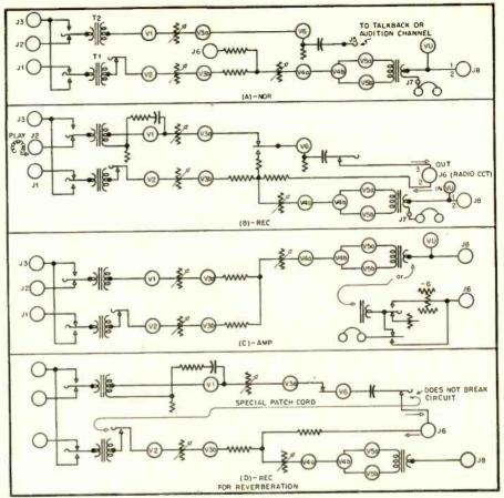
Fig. 4. Block schematic of the amplifier for the three positions of the selector switch,  $SW_{a_a, b, c, d}$ , and when connected for reverberation. When connected to a home music system,  $J_n$  is shorted so the unit is out of the circuit when the selector switch is at NOR.
