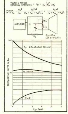
Fig. 2. Calculated curves representing power delivered to  $Z_{\rm m}$  over a range from 1 to 6 ohms, for three values of amplifier resistance  $R_{\rm a}$ .
