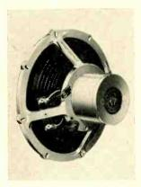
sion of the cone. The Super 5 is supplied mounted on an 8-by-8 in. plywood board with 3½-in.-diameter aperture, which is the effective cone diameter. May be used with two-speaker systems employing 1000-cycle crossover merely by connecting in parallel with the present treble unit and by inserting a 0.5-µf. capacitor in series with the voice coil of the Super 5. British Industries Corporation, 164 Duane St., New York 13, N. Y.
