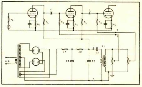
Fig. 3. Typical R-C coupled amplifier with correction network—consisting of C<sub>8</sub>, T<sub>1</sub>, and two potentiometers—arranged to provide cancellation voltages to grids of succeeding stages.
