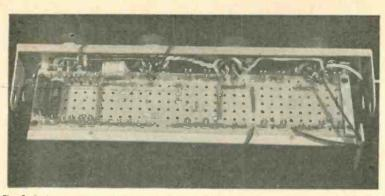
Fig. 2. Resistor mounting card assembled in small chassis with four sockets attached. Terminal lugs may be staked into any desired holes in the board, and thus fit any circuit. Grid and input circuit components are on the top side; plate and decoupling components are located on the bottom.
