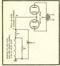
Fig. 15—10. Method for providing the heaters of low-level stages with d.c. R, must be of such value as to keep total bias voltage at correct value; R, keeps heater current at 150 ma.
