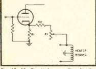
Fig. 15—15. Circuit for cancelling line-frequency hum. A capacitor in series with  $R_2$  can be used for corrective phase shift to bring the phase of the cancelling valtage opposite to that of the voltage being cancelled.
