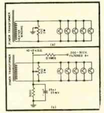
Fig. 15—11. A—Effective circuit for reducing hum resulting from a.c.-operated heaters. B— Elaboration of method shown in A, including positive bias on heater to prevent heater-tocathode emission.
