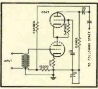
Fig. 9. Schematic of the cascode preamplifier stages in the amplifier section.
