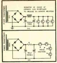
Fig. 15—9. A—Low voltage d.c. heater supply. B—Low current d.c. heater supply. R provides the correct voltage drop for the tube section and Is preferably of the negative-temperaturecoefficient type to protect the heaters from initial current surges.
