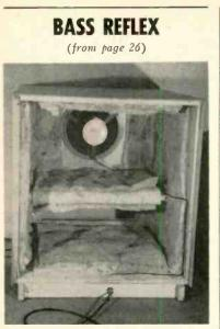
Fig. 3. A horizontal partition was inserted to avoid the raised resonance frequency of a cubical enclosure.
