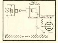
Fig. 15—8. Hum pick-up from the line due to grid-to-earth capacitance.  $C_{\rm T}\equiv$  capacitance between transformer primary and case,  $C_{\rm GR}\equiv$  capacitance between chassis and earth,  $C_{\rm GR}\equiv$  capacitance between grid and earth. For relief,  $C_{\rm GR}$  must be shorted out by earthing the chassis, or the grid must be shielded from earth.
