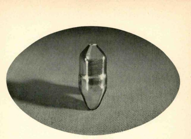
Germanium crystal grown at Bell Telephone Laboratories (life size). It is sliced into hundreds of minute pieces to make *Tronsistors*. Translstor. action depends on the flow of positive current-carriers as well as electrons, which are negative. Arsonic —a few parts per 100,000,000—added to germanium produces prescribed excess of electrons. With gallium added, positive carriers predominate. Latest junction type *Transistor* uses both kinds of germanium in the form of a sandwich.
