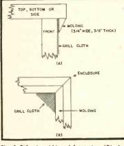
Fig. 4. Side view (A) and front view (B) show how the grill cloth was attached to give a professional appearance.
