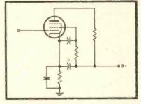
Fig. 15—14. Circuit for cancelling plate-supply ripple and regeneration due to inadequate filtering and decoupling. The value of C<sub>1</sub> in relation to the cathode-to-ground impedance determines the value of the cancelling voltage. (After Wen-Yuan Pan)
