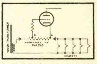
Fig. 15—12. Introduction of hum voltage between grid and cathode due to flow of a.c. return current through chassis.
