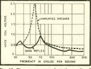
Fig. 10. These two curves show the results of the final bass-reflex enclosure.
