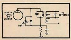
Fig. 1. Where the area is very noisy or the i.f. amplification is insufficient to saturate the limiters with the available signal, two crystal diodes make a very effective additional limiter.
