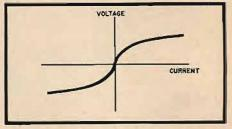
Fig. 2. This curve shows that a disproportionately large current flows through the di-odes when the voltage across them increases beyond a small value. Above that value the diodes effectively short-circuit the discrimina-for transformer of Fig. 1 and provide limiting.
