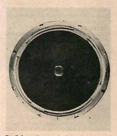
Fig. 7. Spaces between the four original chamois strips are filled with loosely hung chamois to help seal front off from rear air without restricting cone movement.
