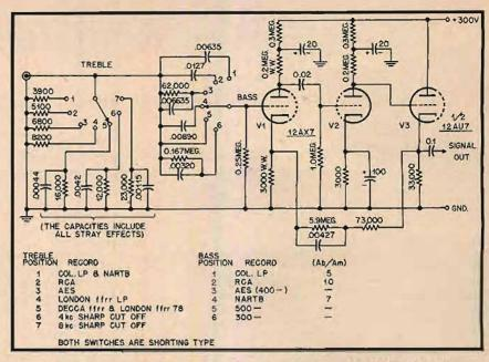
Fig. 5. A complete preamplifier-equalizer, with variable characteristics, designed by the authors in accordance with their method.
