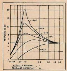
Fig. 2. Relative response of loudspeaker for different values of G.
