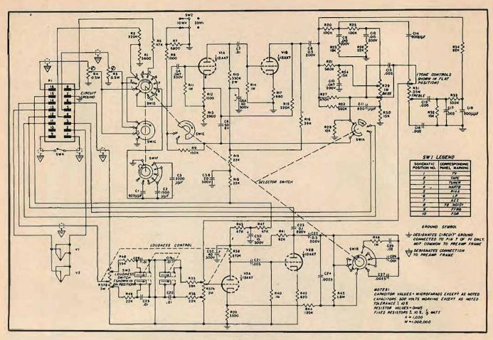
Fig. 3. Complete schematic of the Horizon 5 preamplifier.
