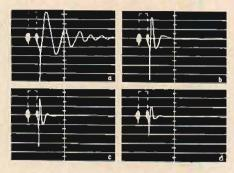
Fig. 7. Sound pressure waveforms showing the effect of amplifier DF on acoustical transient response of loudspeaker system. Solid line shows motion of speaker cone after application of square pulse (dashed line). (a) DF=+0.1, (b) DF=+3, (c) DF= $\infty$ , and (d) DF=-1.2.
