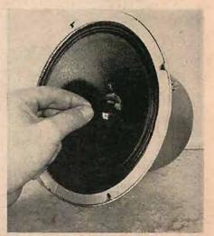
Fig. 3. Inserting shims to hold the voice coil in position.
