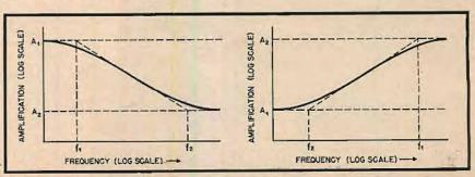
Fig. 6. Additional equalizers with responses as shown are inserted to shift turnover frequency.
