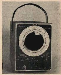
to 5 mv, with a maximum power of 2 watts into a 600-ohm load. Source impedance is under 50 ohms and distortion is less than 0.1 per cent over most of the audio range. Vernier drive provides 14-ins. of scale length per range. Output remains constant within 0.5 db throughout the tuning range. The 512 measures 746 m/s × 64% wx 8"d and weighs 12 lbs. Technical sheet may be obtained from Waveforms, Inc., 323 Sixth Ave., New York 14, N. Y.
