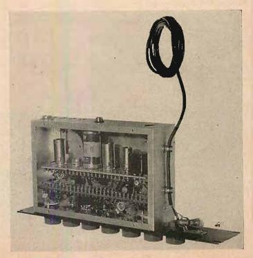
Fig. 8. Photo of the underside shows terminal-board construction.
