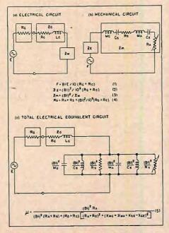
Fig. 1. Electrical and mechanical equivalent circuits of loudspeaker driven by amplifier.
