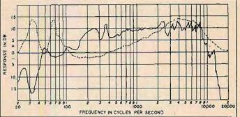
Fig. 8. (left). Sound pressure response of 15-in. coaxial speaker mounted in 8 cu. ft. bass-reflex enclosure with amplifier DF set at + 3. Dotted line represents impedance of speaker. Fig. 9 (right). Sound pressure response of speaker of Fig. 8 with amplifier DF set at - 1.2.
