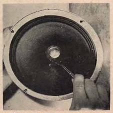
Fig. 2. Removing the dust cover with tweezers.
