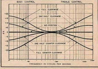
Fig. 3. (left). These curves show the equalization afforded by the various combinations of C1-C2-R1-R2. Fig. 4 (right). The range of tone control available from the circuit.
