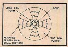
Fig. 5. The spider is cut away except for four sectors which hold it in position while allowing greater compliance.
