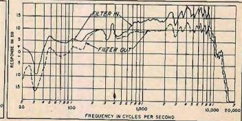
Fig. 10 (left). Sound pressure response of speaker system of Fig. 8 driven by commercial laboratory standard amplifier which has fixed DF of † 10. Compare with Fig. 8. Fig. 11 (right). Sound pressure responses of speaker system of Fig. 8 showing effect of 300-cps filter. Dashed curve is same as solid curve of Fig. 9.
