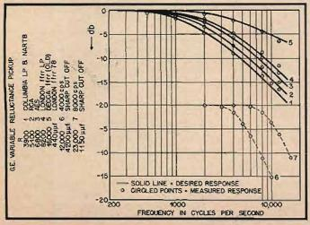
Fig. 4. Various treble rolloffs obtainable from the GE pickup with different values of load resistance. Two sharp cutoffs obtained with loads including paralleled R and C are also shown.
