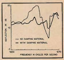
Fig. 2. The effect of resonance on a panel is much decreased when damping material is used as a filler.
