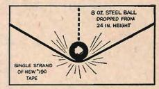
STRENGTH TO SPARE—New 190A tape stands up under even grueling steel ball drop test. Naturally it's tough enough to withstand severe stresses of sudden machine stops, starts and reverses.
