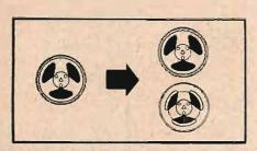
**EXTRA THIN TAPE** – 50% thinner, more potent oxide coating, 30% thinner backing permit more 190A tape to be wound on standard-size reel. Result: one roll of new tape does job of 1½ reels of standard tape.
