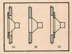
Fig. 3. Common methods of mounting loudspeakers in a wall.
