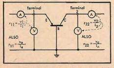
Fig. 1. Equivalent circuit for groundedbase transistor.
