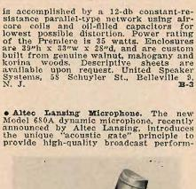
ance throughout an extended frequency range. A peripheral sound entrance channel 2 mils in width, the acoustic gate provides an acoustical resistance loading virtually independent of frequency to the front of the diaphragm, thereby eliminating high-frequency peaks and extending the smooth frequency response over an exceptionally wide range. Altec Lansing Corporation, Dept. AE-6, 9356 Santa Monica Blvd., Beverly Hills, Calif. **B-4**
