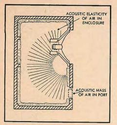
Fig. 10–5. Illustration of mass-elasticity system of bass-reflex Helmholtz resonator, and how it is coupled to the rear of the speaker cone.
