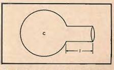
Fig. 9. Diagram of a Helmholtz Resonator.
