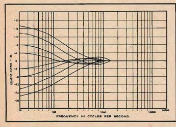
Fig. 1. These curves, taken from a Baxandall tone control, show the overshoot obtained with continuous controls.
