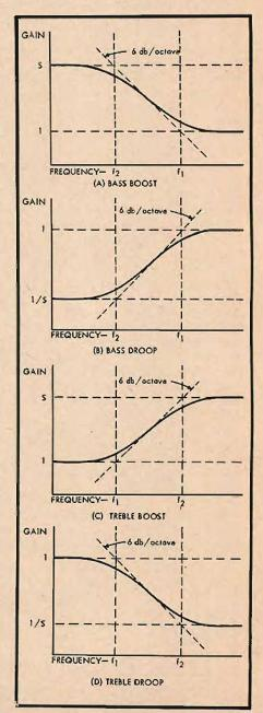
Fig. 8. Generalized curves for the equalizer frequency responses.
