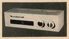
tures include a 10-kc whistle filter, 6 db signal-to-noise ratio at 2.5 microvolts input, and pre-aligned r.f. and i.f. coils. The unit is self-powered and matches other Heathkit models in physical appearance and dimensions. The Heath Company, Benton Harbor, Mich. **B-5**
