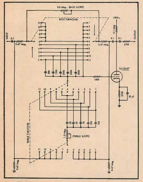
Fig. 4. This form of the tone control gives choice of turnover frequencies as well as control of the bass and treble slopes.
