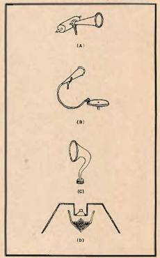
Fig. 10—7. Use of the horn as an acoustical coupler over the last seventy-five years (A) rigidly attached to phono pickup (Edison); (B) attached by flexible tubing (Berliner); (C) curved to conserve space; and (D) folded bass horn with direct-radiator type driver.
