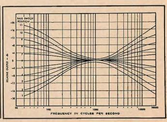
Fig. 2. Curves illustrate the wide range of slope control obtainable with the circuit of Fig. 2. The turnover frequencies are fixed.
