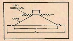
Fig. 1. Typical loudspeaker cross section.
