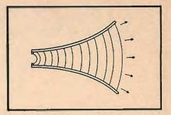
Fig. 10–6. Increase of effective radiating area of a small diaphragm at the throat of a horn to that of the mouth.
