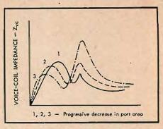
Fig. 12. Varying port area affects the impedance curves for bass-reflex enclosures.
