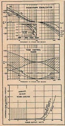
Fig. 1. Performance curves for the Marantz amplifier and Audio Consolette.
