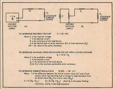
Fig. 3. Two basic constant-current circuits useful for transistor testing.
