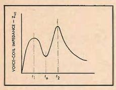
Fig. 11. Impedance curve for the vented box or bass-reflex enclosure.
