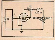
Fig. 4. Pentode vacuum-tube current regulator circuit.
