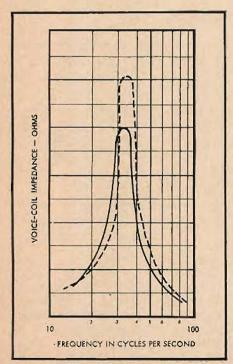
Fig. 4. Voice-coil impedance of loudspeaker in free air (dotted curve) and mounted in wall (solid curve).
