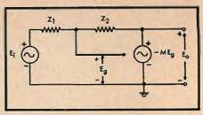
Fig. 5. Equivalent circuit of the tone control.
