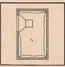
Fig. 5. Cross section of closed box.
