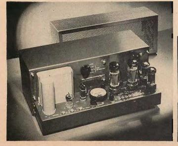
The two Marantz units—Fig. 2 (left) the 40-watt power amplifier with the perforated grille cover removed to show the meter and test switch as well as the adjustable controls. Fig. 3 (below) The Audio Consolette in its wood housing.
