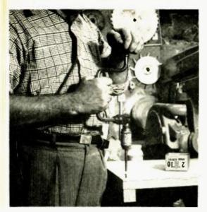
Fig. 8. Glue-screw procedure for firmness is feature of this speaker housing jab. Owner uses brace-operated screwdriver for easier hondling. Note bench is at comfartable working height just belaw bent elbow.
