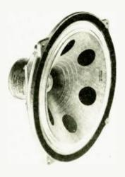
the new Model HP-1214 also incorporates six stabilizing discs of long-stephe fibre which are impregnated into the front of the cone to improve mid-register response, particularly in the 1000-3000 eps range. Lass resonance is 20 eps and ocer-all frequency response is 25 to 14,000 eps. Power rating is 15 watts. Complete information will be supplied on request by Beam Instruments Corp., 350 Fifth Ave., New York 1, N. Y. **M-17**
