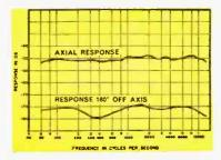
Polar Pattern-Uniform at All Frequencies A-300 cps B-5,000 cps C-10,000 cps Smooth, Peak-Free Frequency Response
