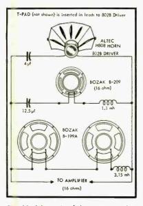
Fig. 11. Schematic of three-way speaker system shows wire-up and values of components. It is also plan of physical placement of speakers within and atop of infinite baffle.
