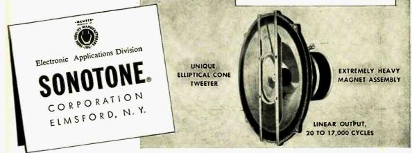
SONOTONE CA-15 COAXIAL SPEAKER has a huge 5-lb. Alnico V magnet, with 15,000 gauss flux density. Unusual velour suspension of the ridged, curvilinear cone drops resonance to 30 cycles, keeps extreme "lows" full, rich and natural. The six-inch non-metallic cone tweeter is elliptical, providing wide lateral dispersion of "highs" without tinniness or piercing effect. 25 watt output, 40 watt peak. Woofer and tweeter also available individually.
