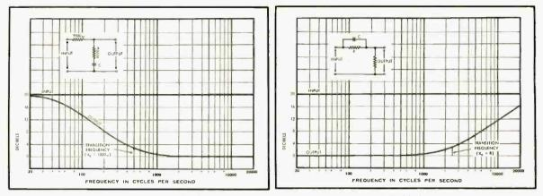
Fig. 6-2 (left). Resistor-capacitor voltage divider, and resulting bass boost. Fig. 6-3 (right). Treble boost circuit.
