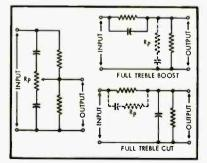
Fig. 6–5. Continuously variable treble tone control. Equivalent circuits for maximum boost and cut are shown, with signicant elements at that point shown in heavy line.
