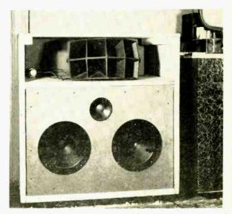
Fig. 5. Bozak assembly in place, with Altec-Lansing tweeter on shelf over. Non-resonant baffle is monolithic Chemstone fitted to framing over gasket, secured with bolts.
