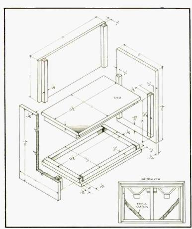
Fig. 3. Isometric view highlights simple building method. Heavy strips are secured to flats as in pallet or skid type construction. They reinforce corners when panels are fitted together. Inset shows placement of Kimsul curtains to eliminate internal standing waves.
