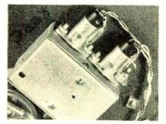
Fig. 7. Close-up showing optional neon indicators and series resistors on each lamp socket.
