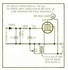
Fig. 2. Basic circuit of thyratron color organ.
