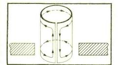
Fig. 4. Voice-coil former with the electrical circuit indicated.
