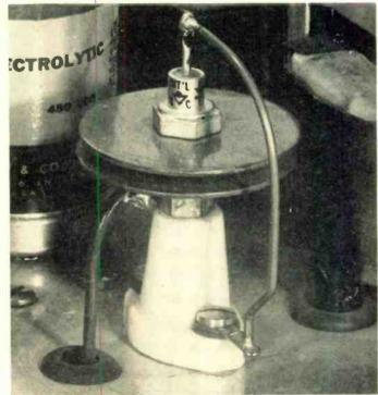
lem of electrical insulation immediately arises. Particularly with power transistors wherein the collector is electrically connected to the case.
