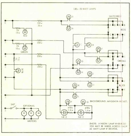
Fig. 9. Alternate lamp circuit used in this model.
