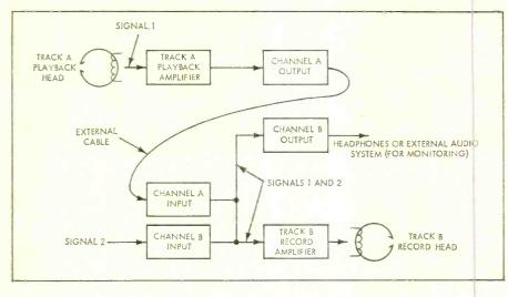
Fig. 2. Sound-on-sound recording with the Model 64.
