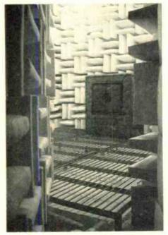
Anechoic chamber in JMI labs for complete acoustical tests of loudspeakers.
