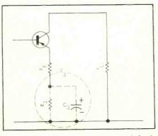
Fig. 26. Common-emitter stage with both a.c. and d.c. series feedback.
