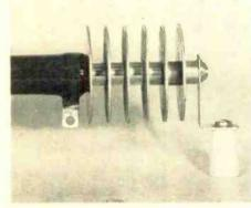
Fig. 4. Experimental cooling assembly.
