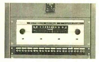
This is the new 314A "Emperor Royale" FM Stereo Tuner. It was designed by Altec to meet requirements for professional use as a monitor and network relay in FM stations. It is shown above in an Altec 13811 Rack Assembly, installed in standard studio relay rack.
