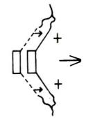
Fig. 11-4. The relationship in a freecone speaker: movement of the diaphragm creates air pressure, or pressure gradient, which promotes particle movement or velocity. ent is derived from the air movement or velocity.
