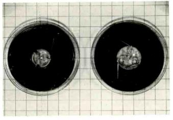
Fig. 2. About ten years ago, the industry increased reel core size from 1.75 inches (left) to 2.25 (right). The loss was playing time but the gain was minimized flutter at the start of play.
