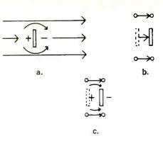
Fig. 11-3. The distinction between velocity and pressure gradient: (A) if the ribbon doesn't move, particle movement in the vicinity creates pressure gradient but not velocity; (B) if the ribbon moves with the air particles perfectly, then there is velocity without pressure gradient; (C) in practice, the ribbon doesn't move as much as the air particles around it, so both velocity and pressure gradient are present.
