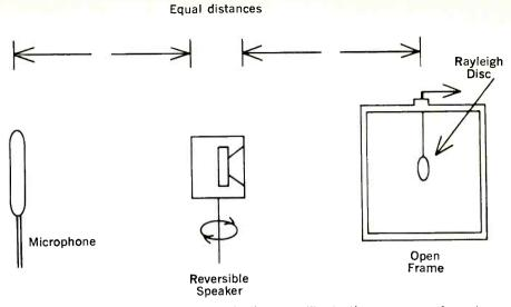
Fig. 11-7. Set-up for using a Rayleigh disc to calibrate the response of a microphone.
