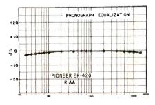
Fig. 7. Accuracy of the magnetic-phono input to the RIAA curve.
