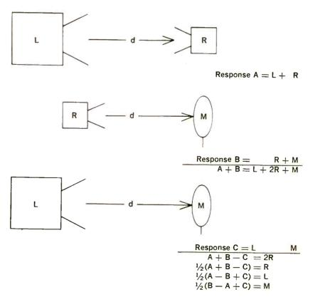
Fig. 11-8. Three measurements necessary for reciprocity test, with the basic calculations necessary to arrive at the microphone and loudspeaker responses. from time to time, as they are subject to change with continued use.
