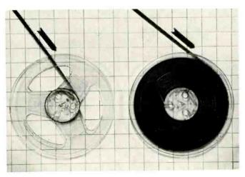
Fig. 1. If the clutch slippage of your take-up reel is poorly adjusted or sticking, the tape pull at the start of take-up (left) can be three times as strong as it becomes later in the take-up cycle.
