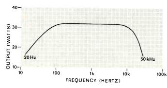
Fig. 2—Power-bandwidth curve showing the limits of frequency response at which the output drops to one-half the rated power.
