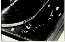
At the left front of the motor board is the speed selector, a plastic lever; adjacent to it is a knurled flat knob which is the vernier speed control, protected by a sliding plastic guard so that once set, it is not likely to be moved accidentally.
