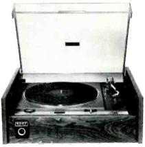
arm, which is static-balanced, is the tubular type with tracking error reported at 1°4′, a stylus force adjustment range of 0 to 3 grams and an acceptable cartridge weight of 4.5 to 11 grams. Its shell is a Universal plug-in
