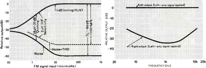
Fig. 3-FM performance characteristics of the NordMende Receiver.
