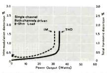
**Fig. 6** – Power bandwidth curve, single channel.
