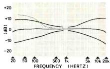
Fig. 3—Tone-control limits, together with the overall frequency response—the center line—with the controls in the "flat" position. The dotted line shows the effect of the loudness/contour control, and filter responses are often plotted on the same graph.
