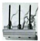
"Wire-wrap" permanent connection technique that eliminates solder joints:
