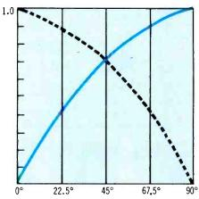
**Fig. 8.** Chart used to determine relative inputs for the five speakers.
