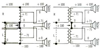
Fig. 2-Dangerous! Short circuit of one amplifier.
