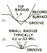
Fig. 7—(A) Illustrates a view of the stylus tip looking down the record groove. In (B), a view of an elliptical tip is shown looking at the record at an angle of 45 degrees (parallel to one groove wall).
