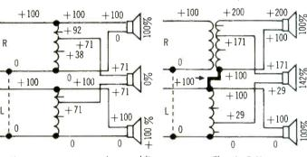
Fig. 1-Wrong! No voltage addition.
