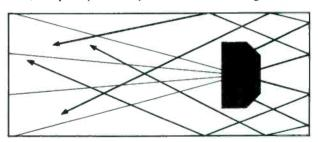
Reflective speakers... these can give a satisfactory illusion of presence and depth. However, these systems require an equalizer for flat response. This in turn generally requires the use of separate (and expensive) preamps and ultra-high-wattage power amps.
