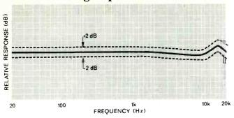
Fig. 4—Tolerance limits of a phono cartridge's frequency response, where solid line is typical response and dotted lines are variations due to manufacturer's quality standards.
