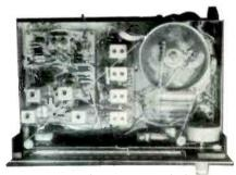
Fig. 2—Open-chassis view of the EICO Model 3200 stereo tuner, showing layout of three major modules.
