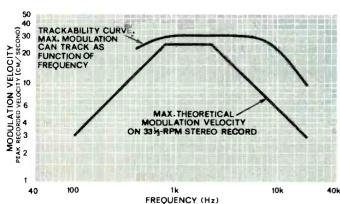
Fig. 3—Frequency response characteristic of phono cartridge with a specification of 20-20,000 Hz ±2 dB.
