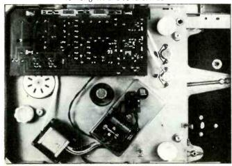
The motor drives the inner turntable through a small belt which isolates motor vibration from the turntable assembly. Below: the stroboscope seen through the window at the front of the panel. The photo was taken at  $33^{1}/_{3}$  rpm, and the line of light below the dots is the position of the 45-rpm dots. A sliding window adjusts for
