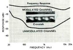
15 to 20 dB separation at 10 kHz.
