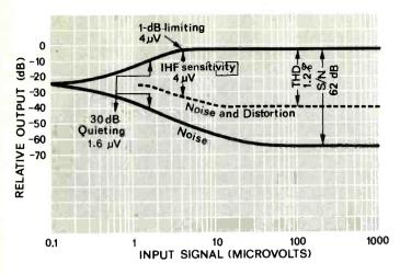
Fig. 3 – FM characteristics of the Model 3200 Cortina
