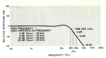
Fig. 5—Frequency-response curve showing several high-frequency limits, depending on how specified.
