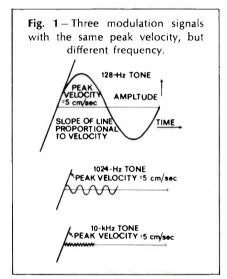
frequency signal. For many cartridges, we would find that there would be little difficulty encountered in reproducing the 1024-Hz tone. A somewhat better cartridge would be required to produce the low-frequency tone also. And an even better cartridge would be needed to reproduce all three signals faithfully.
