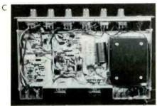
Fig. 2—The rear panel layout of EICO's Model 3150 stereo amplifier is shown in (A). Figures 2B and C show top and bottom views of the chassis, illustrating how duplicate printed-circuit boards are mounted for each channel. Twenty-six silicon transistors, six silicon rectifiers and twelve biasing and protective-circuit diodes are used in this design.
