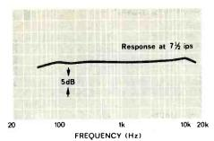
**Fig. 2**—Reproduce frequency response at two speeds of the NordMende 8001/T recorder.
