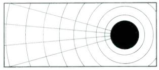
Omnidirectional speakers . . . most are omnidirectional only in the bass range . . . but notice that the vital high frequency tones, regardless of elaborate baffle systems, are perceptible only in a limited listening area.
