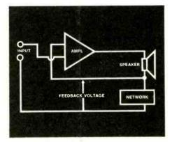
The above circuit illustration shows how feedback voltage is derived when the LWE is connected to amplifier. A voltage is developed and fed back to the same point in the amplifier that the negative voltage feedback enters.
