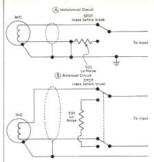
Unbalanced circuits are wired as in Fig. 1A. Balanced circuits are wired as in Fig. 1B. These two circuits assume that low-impedance microphones of 50 ohms are to be used. However, if the impedance of the mikes is of some other low value, the 50-ohm resistor shown must be changed to a value equal to the impedance of the microphone used.
