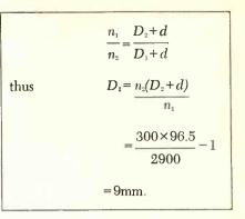
diameter in the above equation, giving So the effective drive at the motor has a diameter of 10mm.
