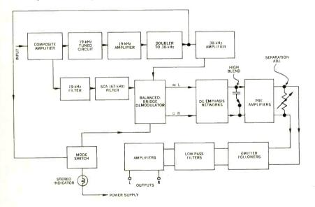
so on, and secondly, to incorporate such convenience features as automatic switching of mode (from monophonic to stereo FM), stereo indicator lights, and the like.
