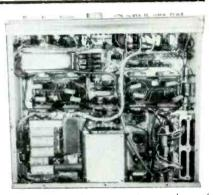
**Fig. 2**—Internal construction makes efficient use of available space, while vertically mounted p.c. boards provide easy servicing.
