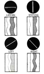
phase signal produces a vertical sweep. Left and right form the arms of an X. The display shows lateral/vertical ratio, channel balance, and level. It is also very useful when cutting mono with a stereo system, as small variations from the lateral mode are easily seen. With an equalizer to produce the RIAA cutting curve, the display will show actual stylus motion.
