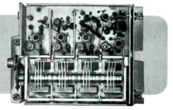
Sansui 4000's new printed circuit design features separate P. C. modules with plug-in multi-connectors for FM MPX, preamplifier and driver amplifiers, permitting faster more economical servicing.
