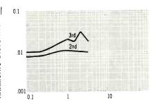
OUTPUT (VOLTS) Fig. 4—Measured harmonic distortion of the IC tone control.
