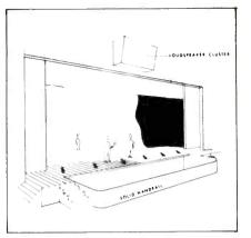
**Fig. 2**—Typical central loudspeaker system with directional footlight microphones.
