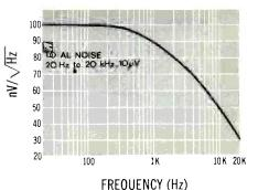
**Fig. 5**—Noise output. Total noise of the circuit from 20 Hz to 20 kHz is 10 μV.
