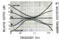
Fig. 3—Frequency-response curves for the tone-control circuit of Fig. 1.
