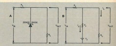
Fig. 1—Zener diode regulation, showing A the actual and B the effective circuit of the zener-controlled power supply.
