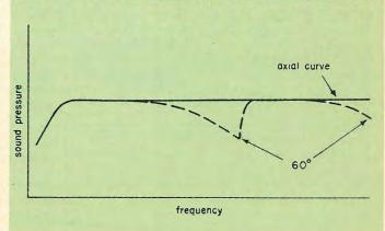
Fig. 1-Two-unit loudspeaker. Nominal frequency response characteristics on axis and at 60 degrees in the plane at right angles to that containing the two units.
