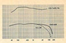
approached. Frequency response measured within  $\pm 2\frac{1}{2}$  dB from 40 to 13,000 Hz in the flat position, while the noise suppressor rolled off response about 10 dB at 10,000 Hz. The autoeject feature was judged useful for those who will use the unit for playing recorded tapes consistently, and it is undoubtedly a convenience in normal use. We had relatively little information about this machine, so everything described or charted is the result of inspection and measurement.
