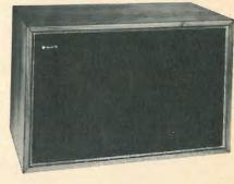
The Criterion 4X speaker system features a four-speaker design, with a 12-in. bass speaker, a 5-in. mid-range, a 3-in. for the 5000-to-10,000 Hz range, and a 1½-in. super tweeter for frequencies up to 20,000 Hz. Impedance: 8 ohms. Size: 22 × 14½ × 11% in. Price: \$69.95.
