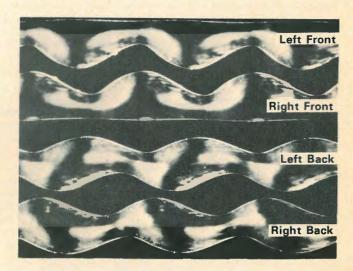
Fig. 2-Magnified view of an SQ record.
