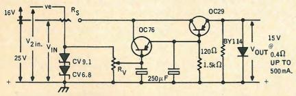
Fig. 5—A simple bench power supply circuit, with rudimentary control, effective over a limited range of values.
