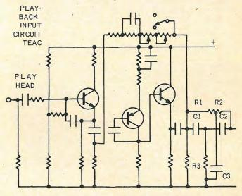
Fig. 3—Playback input circuit (one channel only).
