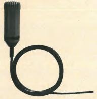
This dynamic microphone uses double-wall construction with two separate cases, one nested inside the other and insulated with highly compliant rubber. The unit weighs 8 oz., is 2% in. long, and has a diameter of less then one in. This omnidirectional microphone has a specified frequency response of 90 to 10 kHz and is matched for low impedance inputs. Price, \$133.
