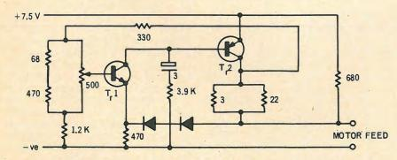
Fig. 6—A variant (by B. R. C. Ltd.) on the supply and motor regulation circuit of the Philips cassette portable shown in the Jan., 1971 issue of AUDIO, p. 28.
