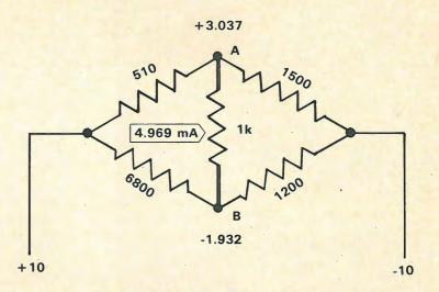
Fig. 2—Bridge with resitances calculated.
