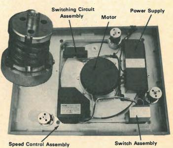
Fig. 1—Underside of the turntable, showing the "black boxes" and the massive isolation mounts consisting of viscous-damped
