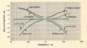
Fig. 9-Frequency response, tone, loudness, and filter characteristics
