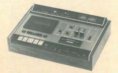
mode it was set for, yet without the tape movement. There are 36 transistors and 30 diodes in the device, and two microphone jacks on the front panel accommodate dynamic mics. Line input and output phono jacks are located on the rear of the walnut-finished cabinet. There are two erase heads—each covering its half of the tape—and one four-track record/play head. The synchronous drive motor
