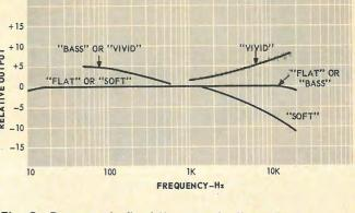
Fig. 8—Response in fixed "tone setting" positions.
