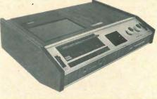
The motor-running signal light indicates green while the machine is in either record or play modes (the record indicator is red, and the overload light is white) as long as the take-up spindle is rotating. At either end of the tape travel (at end of tape or when rewind is completed) the green light dies out, indicating that you should depress the stop key. Thus the stop is not automatic, but the end of tape motion is clearly shown. This indication is effected by a three-transistor circuit.
