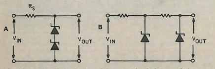
Fig. 3—Where voltage limits are beyond the range of a single zener diode, two or more can be combined, A in series and B in cascade.
