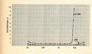
Fig. 7—Distortion vs. frequency at various power levels.
