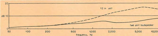
Fig. 3—Directivity of a single 12 in. unit and of a two-unit monitoring loudspeaker having a 7 in. slot in front of the
