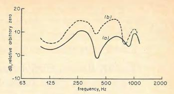
It will be noted that the curve of the directivity of the Fig. 4—Curve a, measured frequency response characteristic of loudspeaker in a corner using warble tone. Curve b, frequency response characteristic of loudspeaker in a corner to be expected as the bass unit is fundamentally omnidirec- calculated from three images in walls and ceilings. (Curves
