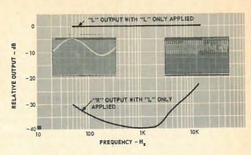
Fig. 4—Stereo FM separation characteristics
