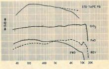
held speed within -2.5 per cent at 85 volts to +0.6 per cent at 135. Frequency response with CrO2 tape was within ±2 dB from 40 to 14,000 Hz in the forward direction, slightly less in the reverse direction. With FeO tape, response was about the same, extending only to 12,000 Hz. With the limiter switch on, response at 10 kHz was down an additional 6 dB.
