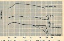
±2 dB from 40 to 12,000 Hz with CrO2 tape and within ±3 dB from 40 to 9500 Hz with FeO tape. The hifilter droops response about 4 dB at 10 kHz with CrO2 tapes, and the curves for FeO tape show the effect of using the hi-filter during both recording and playback modes, showing a droop of 8 dB compared to the 4-dB droop when used in only the playback mode.
