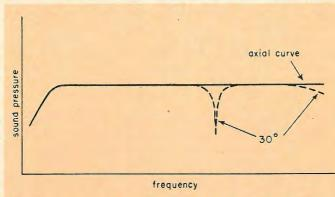
Fig. 2—Two-unit loudspeaker. Nominal frequency response on axis and at 30 degrees in the plane containing the two units.
