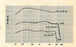
Frequency response with CrO2 tape measured within  $\pm 2$  dB from 40 to 13,000 Hz, with Dolby response differing less than 1 dB at the upper end. With FeO tape, response was within  $\pm 2$  dB from 50 to 9000 Hz, with Dolby response drooping about 4 dB at 9000.
