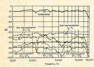
Fig. 7—Intermodulation distortion curves of three-unit monitoring Joudspeaker in free-field room. Sound level 1N÷m2 at five feet from loudspeaker.
