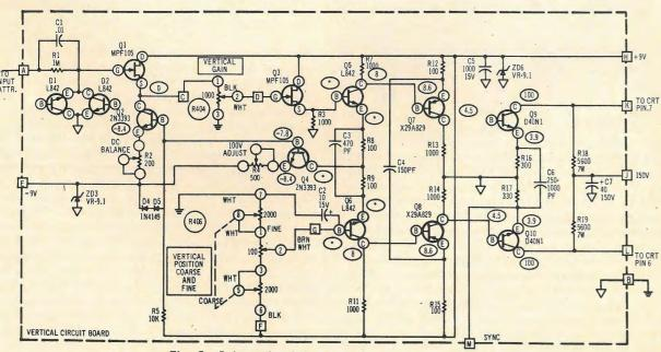
Fig. 3-Schematic of the vertical push-pull amplifier
