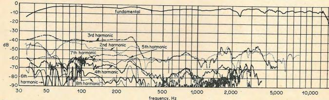
Fig. 6—Harmonic distortion curves of three-unit monitoring loudspeaker in free-field room. Sound level 1N÷m<sup>2</sup> at five feet from loudspeaker
