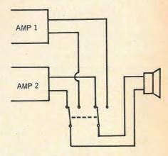
Fig. 1—Amplifier switching system, using two amps and one set of speakers (one channel shown).
