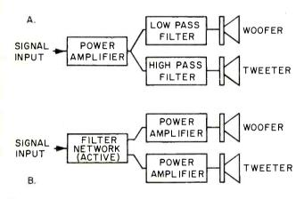
Fig. 1—Possible crossover-amplifier arrangements
