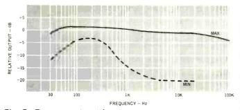
Fig. 5—Tone control and frequency response
