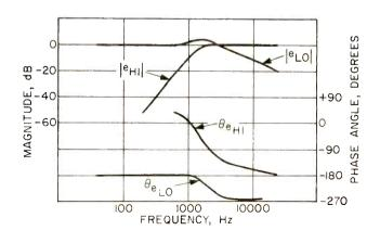
Fig. 3—Measured response of I.C. filter network.
