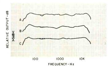
Fig. 1—Response curves with one-third octave pink noise; A is taken on-axis, B at 45 degrees off-axis, and C is an average of five angles.
