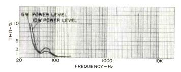
Fig. 3—Harmonic distortion at low frequencies.
