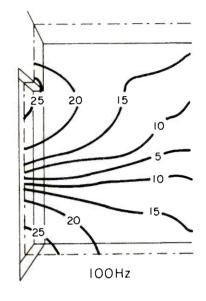
Showing sound field penetrating through a door at 100 Hz.
