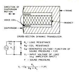
Fig. 1—Equivalent electrical circuit of a dynamic transducer.
