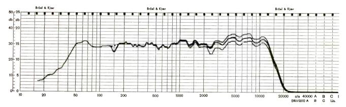
Fig. 2—Frequency response with the tweeter level control in three positions
