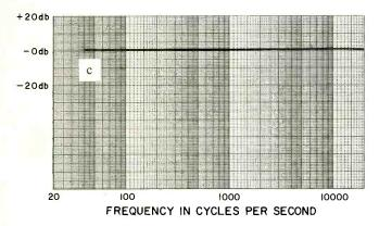
Fig. 3A—Free field axial response of a professional quality omnidirectional dynamic microphone. B, Free field axial response of a professional quality omnidirectional condenser microphone. C, Free field axial response of a ½-in. laboratory condenser microphone.
