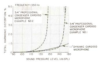
**Fig. 5**—Overload characteristic examples of condenser and dynamic microphones.
