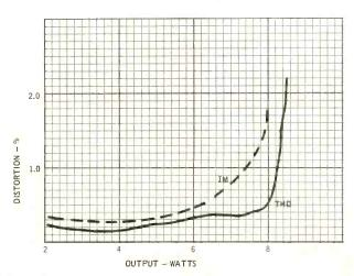
Fig. 4-Power Output, both channels driven (4 ohms)
