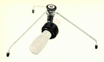
Fig. 9—A typical zero-reflectance mic stand, the Shure S-55P. The mic should be adjusted so that its grille is about 1/8-in. from the floor.
