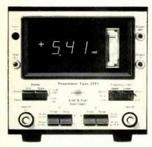
Type 2971 enables frequency response test systems to automatically plot phase response curves, not possible before. The Phase Meter can tolerate 50 dB changes in signal level of both the reference and unknown voltage. Readout is both digital and analog. The 2971 can be used for phase comparison of any repetitive waveform. Price: \$1920.
