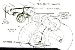
Hall-effect DC motor for absolute speed accuracy, independent of fluctuations in AC line voltage. A second, DC-controlled motor provides the proper hold-back tension. This configuration, standard for professional recording equipment, is responsible for the CR5120's exceptionally low wow and flutter specification of 0.04% WRMS ... performance superior to most reel-to-reel decks.
