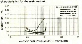
Fig. 4 – Harmonic and intermodulation distortion
