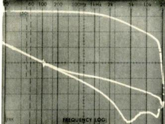
Fig. 4— Stereo separation vs. frequency. Upper trace is the desired output; lower traces show crosstalk to opposite channel with poorer high frequency separation in the *Narrow* i.f. setting.
