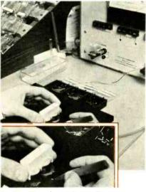
5. Matching of transducers. Electret transducers are measured for capacitance and sorted into matched pairs. This assures accurate channel balance.
