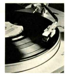
12. All areas of cartridge performance are tested. Tests include frequency response, channel separation, output level, tracking and transient ability. Only cartridges that fully meet published specifications are serialized and placed in stock for shipment.
