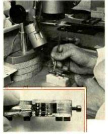
7. Microscopic assembly of complete transduction system. Here, all elastomeric parts are assembled together with transducer elements and positioned by means of three vernier alignment screws.
