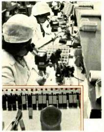
3. Microscopic assembly of damping mechanism. Each elastomeric damper is individually cemented to its own retainer block. Eight dampers are used in each cartridge.
