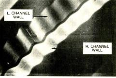
The Same Commercial Recording After 50 Plays With Shure V:5 Type III Cartridge at 1.0 Gram Tracking Force Normal (Inaudible) Wear — Excellent Tracking.
