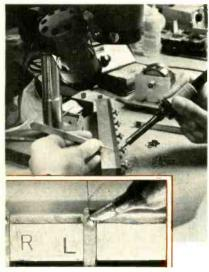
**4.** Microscopic soldering of transducer leads. Two pieces of pure gold wire are soldered to each electret transducer element (negative and positive poles). Thinner than a human hair, this pure gold wire is totally resistant to oxidation, for long, trouble-free cartridge life.
