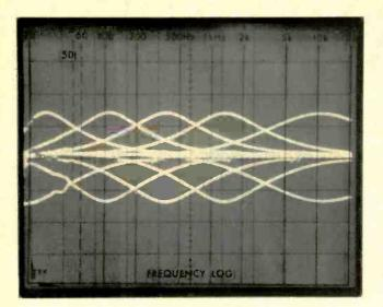
Fig. 7-Control range of the five EQ controls.
