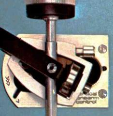
Tracking force is applied with a tempered. flat-wound spiral spring, centered around the vertical pivot. Stylus force remains perpendicular to the record even if the turntable is not level.
