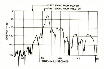
Fig. 10 – Energy-time measurement at one meter on-axis.
