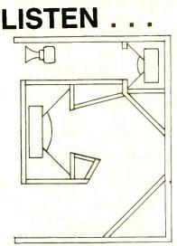
Acoustical Engineering has, for the first time, perfected a single path, exponential bass horn that reproduces fundamentals down to cutoff frequency while remaining small enough to be placed in an acceptably sized piece of furniture. Coupled and properly phased to an outstanding mid-range horn and horn tweeter, the overall response remains constant and produces exceptional clarity and brilliance. Listen ...
