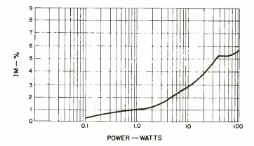
Fig. 9 – IM distortion on  $A_1$  (440 Hz) whem  $E_1$  (41.2 Hz) and  $A_4$  are mixed one-to-one.
