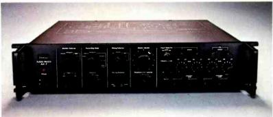
20dB input level attenuators on the 4 main inputs. Reverb is included, as well as circuits for 4-channel, equalization and noise reduction. Record the sounds you create on up to 3 tape decks.
