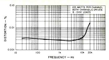
Fig. 11—Harmonic distortion vs. frequency.
