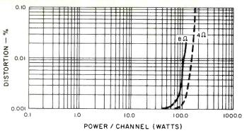
Fig. 10—Power output at 1 kHz vs. distortion.
