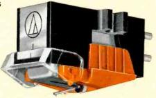
for good reason. Our unique, patented\* Dual Magnet construction provides a *separate* magnetic system for *each* stereo channel. A concept that insures excellent stereo separation, while lowering magnet mass. And the AT12XE features a tiny 0.3 x 0.7-mil nude-mounted elliptical diamond stylus on a thin-wall cantilever to further reduce moving mass where it counts. Each cartridge is individually
