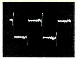
Fig. 2 — Response to 1-kHz square wave.
