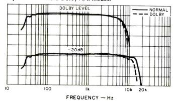
Fig. 2—Record/playback response of Scotch Master III FeCr tape in Normal and Dolby N/R modes.
