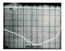
Fig. 5—Frequency response and channel separation in the FM narrow-band mode.
