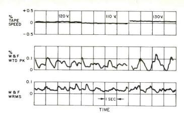
Fig. 5—Tape speed vs. line voltage and flutter.
