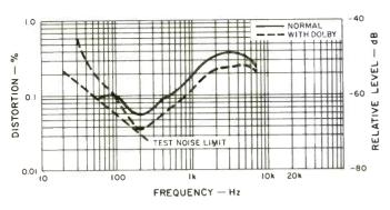
Fig. 5—Third harmonic distortion vs. frequency for normal and Dolby modes at 10 dB below Dolby level (200 nWb/m) with Scotch Master III FeCr tape.
