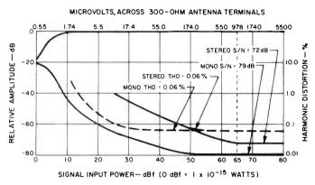
Fig. 6—Mono and stereo quieting and distortion characteristics.
