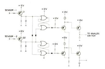
Fig. 2—Function selector network.
