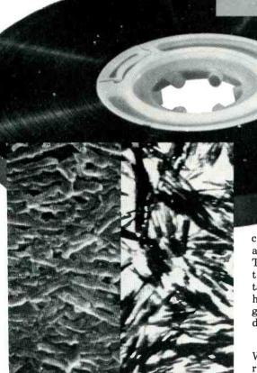
TDK SA tape surface left) enlarged 30,000 times. TDK Super Avilyn particles (right) enlarged 20,000 times.
