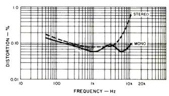
Fig. 7—Harmonic distortion vs. frequency, mono and stereo FM.
