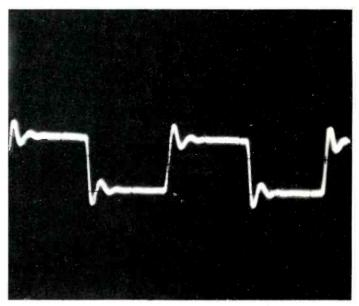
Fig. 2 — Response to 1-kHz square wave.
