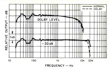
Fig. 2—Frequency response with TDK SA.
