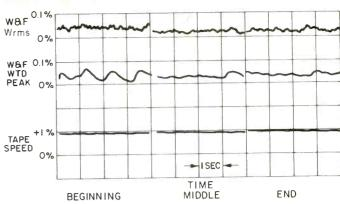
Fig. 6—Tape speed variation and wow & flutter measured at the beginning, middle, and end of a cassette.
