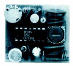
he DNR device is essentially a dynamically controlled LPF that is inexpensive, simple and compact in implementation, and reasonably free of audible side effects.
