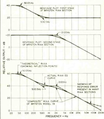
Fig. 1—RIAA equalization in the Bryston 1B preamp is accomplished in two separate stages (upper
