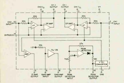
Fig. 3—Block diagram of the LM1894.
