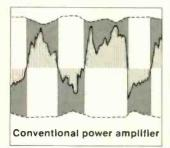
Solid line: audio output signal Broken line: power supply voltage Shaded area: wasted power Vertical lines: power to speakers
