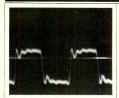
Fig. 2—Square wave response, P22S cartridge.
