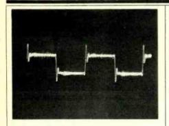
Fig. 2—Response to 1-kHz square wave.
