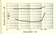
Fig. 3—Response of left channel and separation.
