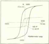
High coercivity and high magnetic flux density for high magnetic energy.
