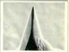
Fig. 1—Lateral SEM view of the van den Hul stylus in the MIT-1. The dark area in the center of the stylus, from the tip to where it begins to widen, is the actual groove contact area, which is 143  $\mu$  long by 10  $\mu$  wide. (x300 magnification.)
