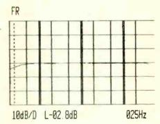
Fig. 4—Highlevel input frequency response was down 0.3 dB in left channel and 0.4 dB in right channel at 40 kHz.
