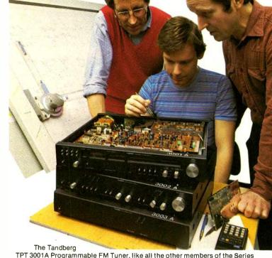
TPT 3001A Programmable FM Tuner, like all the other members of the Series 3000A, features discrete components — not integrated circuits — individually selected to meet ideal performance parameters.
