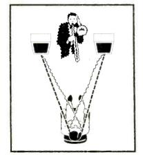
Stereo speakers produce two sound arrivals at each ear. confusing the ear-brain center and diluting the image.
