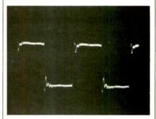
Fig. 2—Response to a 1-kHz square wave.
