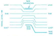
Fig. 1—How companding works.
