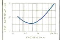
Fig. 3—Hearing thresholds above white noise for pure tone.
