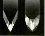
Each Signet TK10ML MicroLine stylus is created from a whole, natural octahedral diamond, oriented for longest life, and with a square shank to precisely fit the laser-cut hole in our unique, ultra-rigid low-mass boron cantilever. You get perfect alignment. Period
