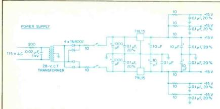
Fig. 6—Schematic diagram of the power supply. Note separate power feeds for each channel, to reduce crosstalk.
