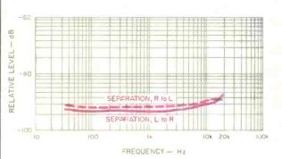
Fig. 3—Separation vs. frequency.
