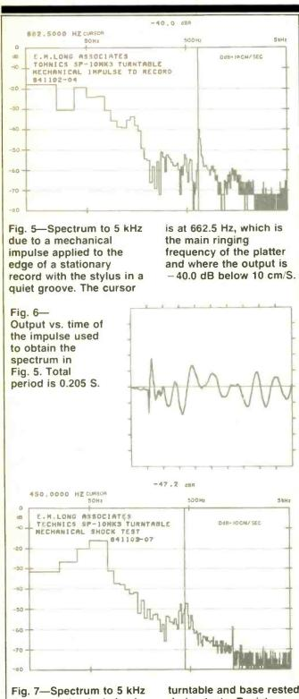
Fig. 7—Spectrum to 5 kHz due to mechanical shock applied to the massive platform upon which the
