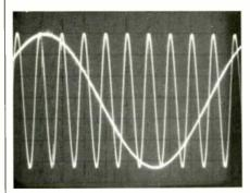
Fig. 8—Phase error check using tones of 200 Hz (left channel) and 2 kHz (right channel).
