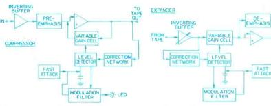
Fig. 2—Block diagram of the compressor section.
