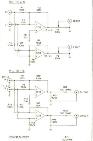
Fig. 3—Schematic diagrams for an active M-S matrix: Right-left to M-S encoder (top), M-S to right-left decoder (center), and power supply (bottom). Capacitors C5 and C6, shown in the power supply, should be mounted as close as possible to IC1 and IC2 and should be used even if a different power supply is connected.
