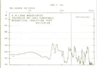
Fig. 9—Spectrum to 100 Hz due to a 100 dB SPL acoustic field at the record surface with the stylus in a quiet groove near the middle of a stationary record. The acoustic isolation is excellent.
