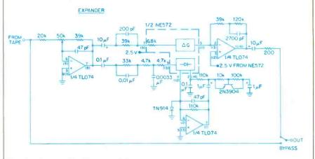
Fig. 5—Schematic diagram of the expander section.
