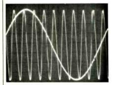
Fig. 8— Twin-tone phasetest signals (200 Hz and 2 kHz) showed negligible phase shift in CD player section.
