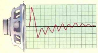
The illustration shows a conventional cone "ringing" long after the electrical impulse from the amplifier has ended. It's known as Time/Energy distortion.
