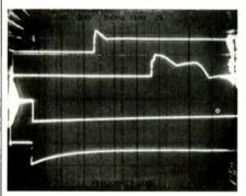
Fig. 3—Response of ALC to sudden 10-dB level changes. Upper two traces show reaction of ALC to 10-dB rise in slow (top) and fast modes; displacement of fastmode curve to the right is a triggering error, not a delay in ALC action. (Scales: Horizontal, 0.1 S/ div.: vertical, 10 dB/div.) Lower two traces show reaction of ALC to 10-dB drop in slow and fast (bottom) modes; note the very gradual recovery rate in slow mode. See text. (Scales: Horizontal. 5 S/div.; vertical, same as upper traces.)
