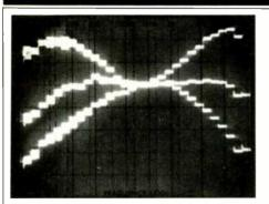
Fig. 4—Range of playback tone controls, showing maximum boost (top trace), maximum cut (bottom trace), and "flat" (middle trace). Response of playback speaker/ headphone amp could not be flattened further than shown. See text. (Scale: 5 dB/div.)
