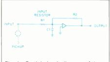
Fig. 1—Partial circuit diagram of the MC-2 pre-preamp.
