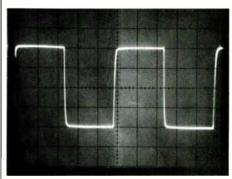
Fig. 2—Response of 3009A amplifier to a 20-kHz square wave, at 200 watts into 8-ohm load. (Scales: Horizontal, 10 μS/div.; vertical, 20 V/div.)
