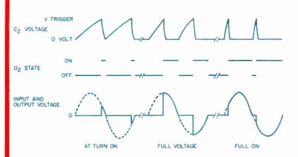
Fig. 2—Timing diagram. Transistor Q1 (not indicated) turns on when C2's voltage (upper trace) is higher than Q1's trigger voltage; this discharges C2. Transistor Q1 also triggers triac Q2 (middle traces), which delivers voltage to the output (lower trace). The output-voltage buildup is best seen by comparing the "on" times of Q2 with the output (solid lower trace) just below it; the dashed lines show input from the a.c. line.
