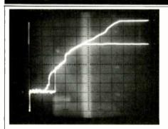
Fig. 2—Effect of a sudden increase in the level of a 1-kHz input signal, with ALC (fast mode) and without it. Note how ALC limits the signal at 50 dB above the tape noise level, while, without ALC, the signal rises 25 dB further. See text. (Scales: Vertical, 10 dB/div.; horizontal, 2 S/div.)
