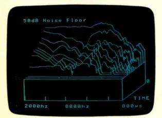
Computers provide information that conventional tests cannot. The display above shows how the various frequencies the driver produces fade away after the signal is cut off.
