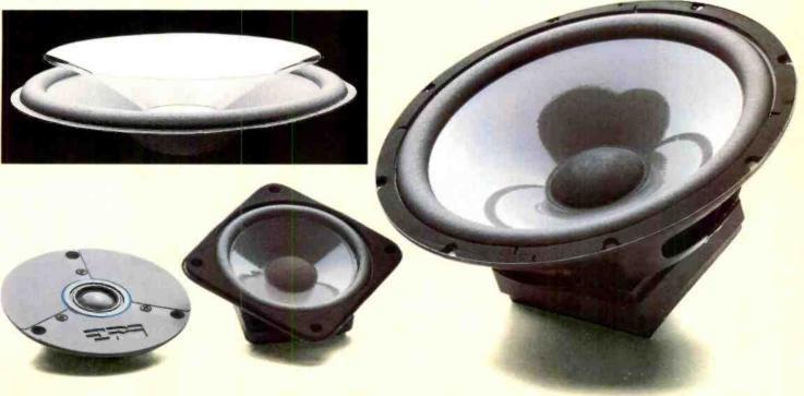
The cone layers are bonded together with a lamination process developed by EPI. The composite cone material has an ideal combination of stiffness and lamping.
