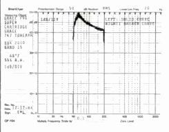
Fig. 2—Low-frequency tonearm/cartridge resonance is at 6 Hz, with a Q of 4.6, using B & K 2010 test record.
