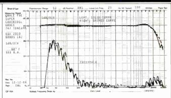
Fig. 1—Frequency response and interchannel crosstalk of arm and cartridge, using B & K 2010 test record. Note unusually close matching between channels.
