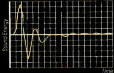
A speaker with a T/E technology cone stops producing sound almost immediately after the signal ends.
