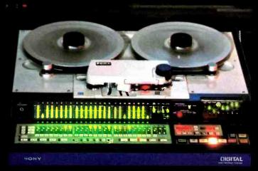
Sony PCM-3324 Multitrack Recorder for professional use.
