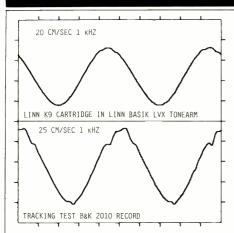
Fig. 11—Tracking test of K9 cartridge in Basik LVX arm shows very little jitter, which indicates good stability. The mistracking in the lower graph is with the highest level band of B & K 2010; the performance is guite good.
