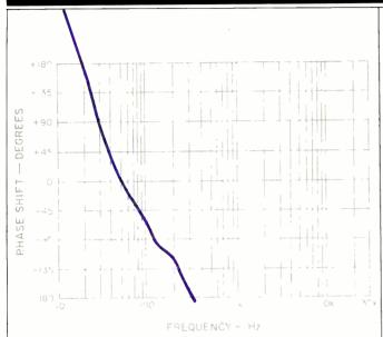
Fig. 5—Acoustic phase response for 193-Hz crossover, measured at 1 meter with speaker placed on floor.
