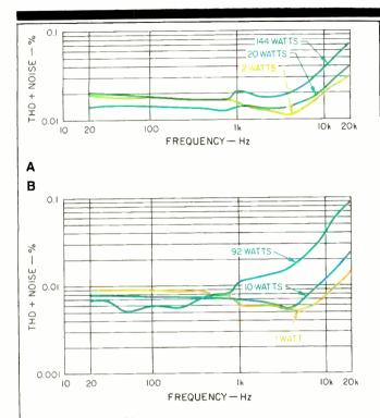
Fig. 1—THD + N vs. frequency for 4-ohm (A) and 8-ohm (B) loads.
