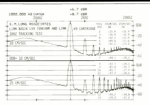
Fig. 12—Spectrum analysis of the cartridge output when reproducing the test tones of Fig. 11. The third harmonic (at the
