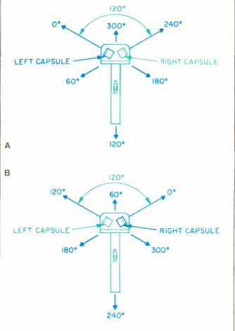
Fig. 1—Capsule layout of the AT-9400. The angles for the left capsule (A) correspond to the response curves shown
