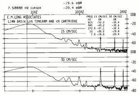
Fig. 15—Spectrum analysis of distortion products from signals shown in Fig. 13. Note that the frequency range
