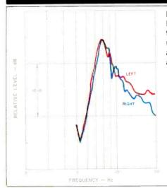
Fig. 3— Low-frequency tonearm/cartridge resonance peaks at 8.0 Hz with a Q of 5.7.
