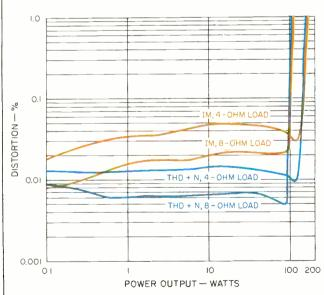
Fig. 2—THD + N at 1 kHz, and SMPTE IM, both vs. power output.
