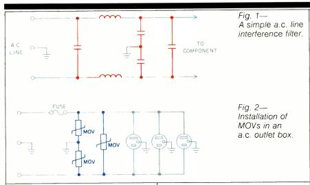
zeners, thyristors, or varistors should be placed across the a.c. line and between a.c. lines and ground. A high-power zener network can be located across power-supply secondaries or between rectified outputs and ground. A heavy-duty solution to recurring problems is the installation of a constant-voltage transformer, which can minimize the effect of both surges and sags. Isolation transformers provide an ideal way to protect equipment from power fluctuation.
