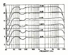
Fig 1—Analog-tape output curves for six recording levels. Note how high-frequency roll-off above 8 kHz increases with recording level. Recordings were made at 15 ips; kink in curves between 100 and 200 Hz is an artifact of the measuring system (Data taken from John Borwick, Sound Recording Practice, Oxford University Press, London, 1976, pg. 119.)
