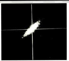
Fig. 8—Interchannel phase difference, using pink noise from B & K 2011, band 7.
