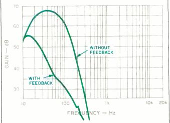
Fig. 2—Amplifier frequency response, measured from left input to speaker terminals, with feedback loop both connected and opened.
