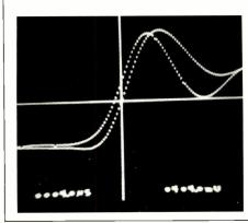
Fig. 10— Time delay between right and left channels. Right channel leads left by 4.0 μS.
