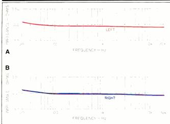
Fig. 2—Impedance of left (A) and right (B) capsules. The two curves are virtually identical, and impedance (920 ohms at 1 kHz) is lower than the rated 1.5 kilohms. Note that impedance scale is logarithmic.
