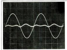
Fig. 3—THD at 1 kHz for 10 watts output into 8-ohm load. Large trace is output signal; small trace is distortion residue after subtracting input frequency.
