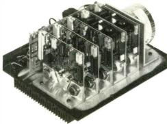
They are frequencydriven and provide dynamic soft clipping for overload protection. The bass amplifler is rated at 100 watts RMS power; the satellite amps at 80 watts RMS per channel. THD is less than 0.01%.
