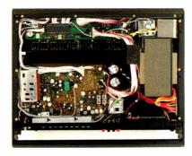
A glimpse inside reveals how carefully thought-out the R4 is. No space is wasted. Electronic circuitry, heat sinks, transformers, etc., are all contained within a box that stands only 23/4" high.
