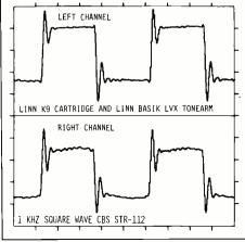
Fig. 16— Response to 1-kHz square wave, using CBS STR-112 test record.
