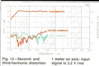
third-harmonic distortion level vs. frequency for 90 dB SPL output at signal is 3.2 V rms (2.5 watts).
