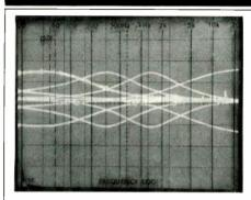
Fig. 3—Boost and cut range of equalizer controls. Sweep is logarithmic, from 20 Hz to 20 kHz. Vertical scale: 10 dB/div.
