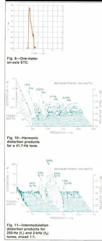
appeared distorted on an oscilloscope monitoring the signal coming from a high-intensity microphone (whichever occurred first). At each frequency, the maximum peak input voltage and the corresponding generated peak output sound pressure level at 1 meter were recorded.
