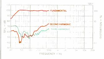
Fig. 13—Same as Fig. 12input signal of 10 V rmsbut for 100 dB SPL at(25 watts).1 meter on axis, using
