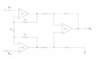
Fig. 5B—The topology of an instrumentation amplifier offers high accuracy and a common-mode rejection ratio exceeding 100 dB. Here, output voltage is:
