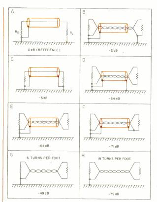
Fig. 6—Relative susceptibility of common cabling circuits to electricfield and magnetic-field coupling.
