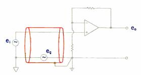
Fig. 3A—An op-amp used as a single-ended amplifier. The distinguishing feature of the singleended configuration is the through connection of the zero-signal reference conductor, which means that ground-line signals ( $e_g$ ) will be amplified. As a result, the output voltage for the single-ended amp equals the gain, A, multiplied by the sum of the input and ground voltages:
