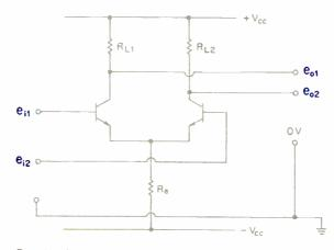
Fig. 2—A commonly used differential amplifier configuration, often known as a long-tailed pair.
