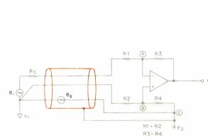
Fig. 5A—An op-amp connected as a differential amplifier can reduce sensitivity to ground-line signals. However, common-mode rejection is seriously degraded by signal-source resistance ( $R_s$ ). Output voltage in this setup is:
