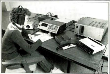
In the National Bureau of Standards' parallel listening tests, subjects were asked to pick out which of two recordings had been encoded with the Copy-Code notch, by reference to a third, unencoded recording. The average percentage of correct identifications was 62.3%
