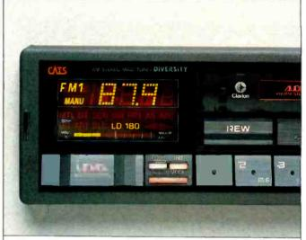
noise reduction are both available, and tape equalization (70- or 120-μS) is selected automatically. I especially liked the way the stop/eject button operates. If you push this button once, the tape stops playing but remains inside the unit. Push it a second time, and the tape pops out.
