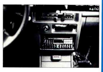
The dashboard radio slot was gradually enlarged to be a snug fit for the new Alpine electronics.
