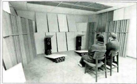
The NBS listening room used soundabsorbing materials on the wall behind the speakers, on the side walls, and on the ceiling; sounddiffusing panels were used on the fourth wall (not shown). Only two subjects were allowed to listen at a time.
