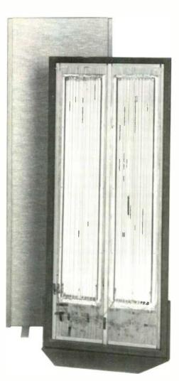
The original Magneplanar' prototype in foreground (utilizing aluminum foil strips on a mylar diaphragm).
