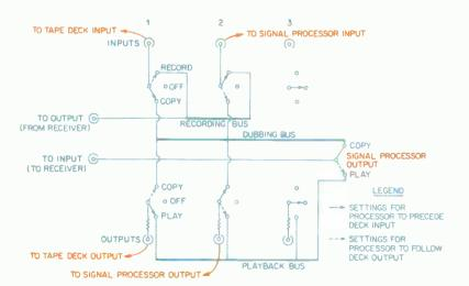
Fig. 6—Using this setup, a signal processor can be used to modify the signal going to a tape deck in recording (solid arrows) and to modify the signal coming from the deck in playback (dashed arrows).
