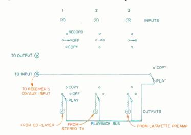
Fig. 2—The switchbox connections and settings now used by the author. (Wiring paths to switchbox elements not in use have been emitted for clarity.) No significant loading effects have been observed from this arrangement. To add still more inputs, signals could be fed to the jacks at the top of the diagram; all switches would then be set to "Copy." See text.
