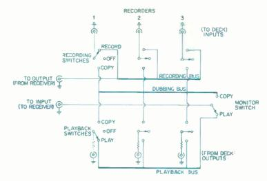
Fig. 1-Circuit of the Russound TMS-3 tape switchbox.
