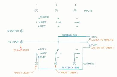
Fig. 3—Connections and settings used to compare two tuners or other high-level sources.
