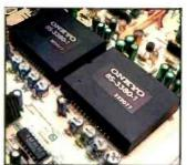
Most of our models also benefit from Opto-Coupling, an Onkyo-developed technology that transmits data optically rather than through conventional wiring for more accurate CD sound.
