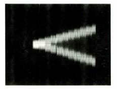
Fig. 10—Monotonicity test shows an almost perfect, symmetrical "staircase" display.
