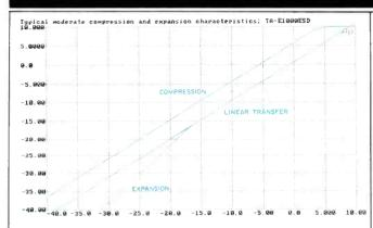
Fig. 5—Typical compression and expansion characteristics of Sony TA-E1000ESD, superimposed on linear transfer curve. Input levels are shown on horizontal axis, output levels on vertical axis; see text
