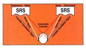
Each Polk SDA incorporates a special extra set of drivers which radiate a difference signal that cancels the undesirable signal going from the wrong speaker to the wrong ear (interaural crosstalk distortion).
