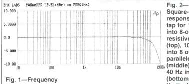
Fig. 1—Frequency response for 8-ohm loads on the 8-ohm taps.
