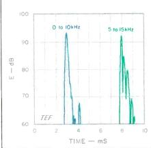
Fig. 3— On-axis energy/ time curves over standard range (left) and centered over tweeter range (right). Tweeter ETC has been shifted right by 5 mS, for clarity; see text.
