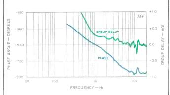
Fig. 2—Phase angle and group delay.
