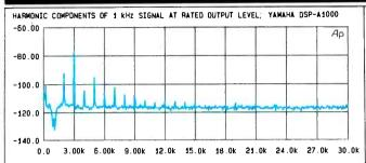
Fig. 5—Spectrum analysis of harmonics of 1-kHz main-channel signal at 80 watts per channel into 8 ohms. Curve shown is averaged result of 16 acquisitions, to reduce displayed noise and improve display of coherent signals.
