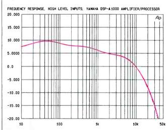
Fig. 2—Frequency response of effects channels in "Concert Hall 2" mode, for line input signal. Curves have been smoothed to eliminate time-delay effects; see text.
