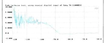
Fig. 7—Fade-to-noise test of D/A converter section.
