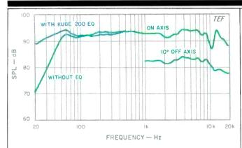
Fig. 1—Equivalent 1-meter frequency response.
