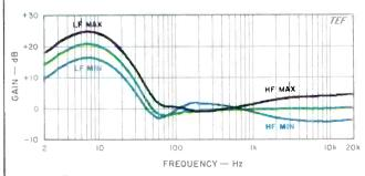
Fig. 8—Frequency response of KUBE 200 equalizer at different control settings.
