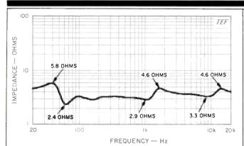
Fig. 9—Magnitude of impedance vs. frequency.
