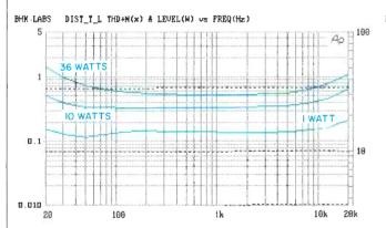
Fig. 3—THD + N (solid curves) and power output (dashed curves) vs. frequency, with 8-ohm
