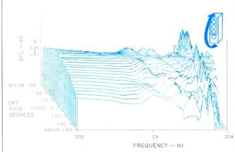
Fig. 5—Vertical off-axis response, normalized to the on-axis response; see text.
