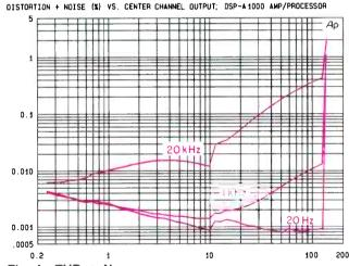
Fig. 4—THD + N vs. power output per channel into 8-ohm loads for main channels (A) and center channel (B).
