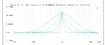
Fig. 4—Range of slopes that can be assigned to any of the three parametric equalizer bands, at maximum boost setting. Slopes for maximum cut setting were identical.
