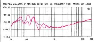
Fig. 6—Spectrum analysis of main-channel residual noise for 1-watt output with 500-mV line-level input.
