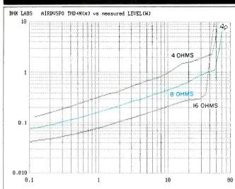
Fig. 5—THD + N vs. power for various loads on 8-ohm tap.
