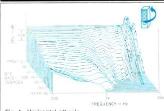
Fig. 4—Horizontal off-axis response, normalized to the on-axis response; see text.
