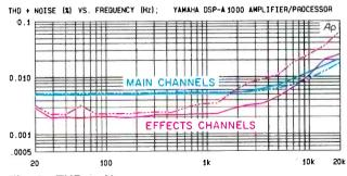
Fig. 3—THD + N vs. frequency for main and effects outputs at rated output into 8-ohm loads, for left channels (solid curves) and right channels (dashed curves).
