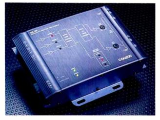
The DA-55 utilizes a U.S. made Dual Single-Bit Chip Set design with 18-Bit Resolution, which incorporates a Dual 8 Times Oversampling Digital Filter, a 64 Times Oversampling Fifth Order Delta-Sigma Modulator, as well as an Ultralinear Digital to Analog Filter Set (a Fourth Order Butterworth Switched-Capacitor Filter with multiple feedback loops followed by a Second Order Butterworth Analog Filter). The Filter
