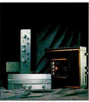
Our new "classic" power amplifier had to be a mono-block; separate audio circuitry, power supply, even power transformer and chassis. Monaural amplifiers maximize stereo separation, eliminate crosstalk and lead to perfect imaging.
