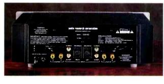
Three sets of inputs and proprietary output binding posts give the D240 complete flexibility in connection to your music system.
