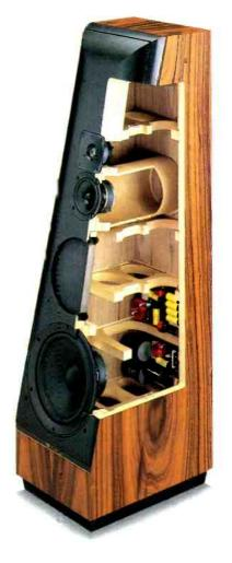
The baffle is sloped to properly position the drivers for correct time alignment and accurate reproduction of transient musical information. It also incorporates rounded edges to greatly reduce energy diffraction which contributes to very "open" reproduction.
