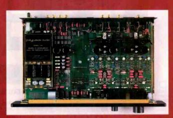
DIGITAL INPUTS Yes the 940 can be configured with Direct Digital inputs, with the optional 20-bit, 8 times oversampling DAC module, providing both coax and optic inputs. This is the same converter module which is the heart cf our highly acclaimed models 300 and 900 off board DACs.
