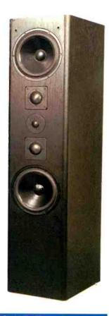
The Diablo Model 2 is a floor-standing, three-way, sealed-box speaker. Arrayed in a D'Appolito configuration, the five drivers include two 10-inch long-throw woofers, two titanium-dome midranges, and one titanium-dome tweeter. Rated anechoic frequency response is 35 Hz to 26 kHz, ±3 dB; typical in-room bass response is 3 dB down at 26 Hz. Sensitivity is 87 dB; nominal impedance is 4 ohms, minimum 3 ohms. Price: \$9,000 per pair.
