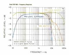
Fig. 2---Center- and surround-channel responses, RSP-980. For clarity, surround-channel curve has been lowered by 0.5 dB.
