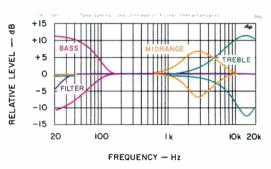
Fig. 2—Tone control and infrasonic filter characteristics.
