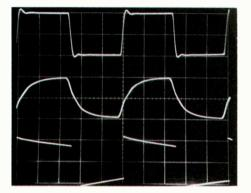
Fig. 2—Square-wave response for 10 kHz into 8-ohm load (top), 10 kHz into 8 ohms paralleled by 2 µF (middle), and 40 Hz into 8 ohms (bottom).
