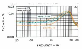
Fig. 3—THD + N vs. frequency at 0 dBFS.
