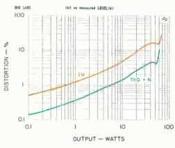
Fig. 3—THD + N at 1 kHz and SMPTE IM distortion vs. power output, for 8-ohm loads on the 8-ohm tap.
