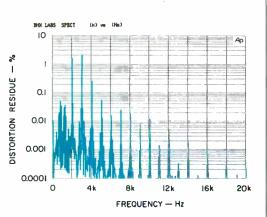
Fig. 6—Spectrum of harmonic-distortion residue for a 1-kHz signal at 10 watts out into 8 ohms.
