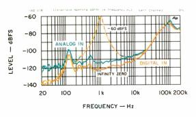
Fig. 7—Spectrum analyses for "infinity zero" signals and 1-kHz tones at -60 dBFS.
