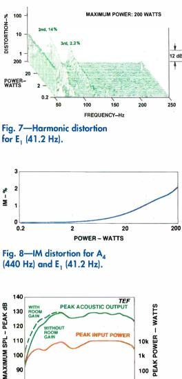
PEAK POWER 100 1k 90 100 80 10 10k 20k 20 100 1k FREQUENCY - Hz Fig. 9—Maximum peak input power and sound output.
