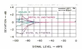
Fig. 5—Linearity error vs. level at 1 kHz.
