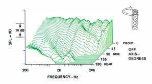
Fig. 3—Horizontal off-axis frequency responses.
