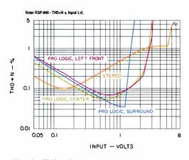
Fig. 4—THD + N vs. input voltage, RSP-980.
