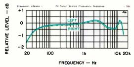
Fig. 2—Frequency response, FM tuner section.
