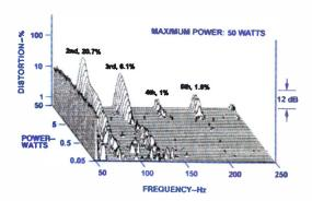
Fig. 7—Harmonic distortion for E<sub>1</sub> (41.2 Hz).
