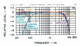
Fig. 5—Frequency response, Dolby Pro Logic mode.
