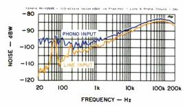
Fig. 4—Noise analysis, stereo mode.
