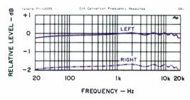
Fig. 7—Frequency response, D/A section.
