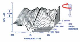
Fig. 3—Horizontal off-axis frequency responses.
