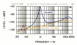
Fig. 12—Noise analysis, D/A section.
