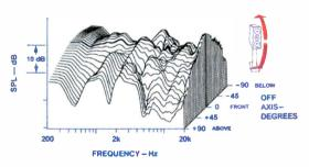
Fig. 4—Vertical off-axis frequency responses.
