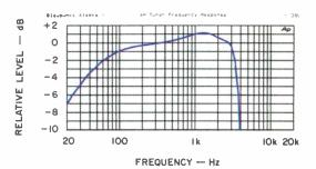
Fig. 5—Frequency response, AM tuner section.
