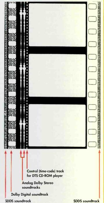
DTS: The compressed soundtrack from Digital Theater Systems actually emanates from a separate CD-ROM player, but it is controlled by a synchronizing time code optically printed on the film and read by a head on the projector. The time code can be seen as a series of vertical dashes just to the right of the two analog tracks.
