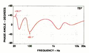
Fig. 5—Impedance B magnitude (A) and phase (B).
