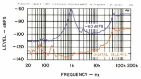
Fig. 11—Noise analysis, D/A converter.
