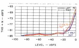
Fig. 8—THD + N vs. level, CD section.
