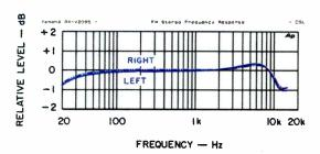
Fig. 15—Frequency response, FM tuner section.
