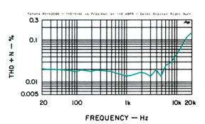
Fig. 14—THD + N vs. frequency, worst channel, Dolby Digital mode.
