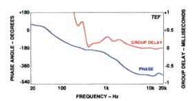
Fig. 2—On-axis phase response and group delay.
