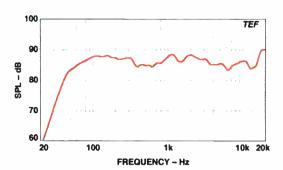
Fig. 1—On-axis frequency response.
