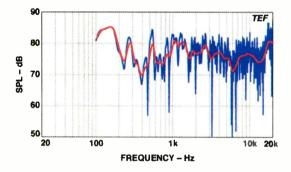
Fig. 6—Three-meter room response.
