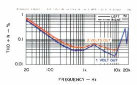
Fig. 7—THD + N vs. frequency, CD section.
