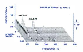
Fig. 8—Harmonic distortion for A<sub>2</sub> (110 Hz).
