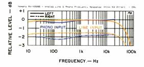
Fig. 3—Frequency response, stereo mode.
