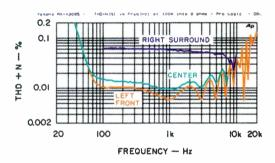
Fig. 6—THD + N vs. frequency, Dolby Pro Logic mode.
