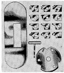
Molding cutterhead knives, table insert.
