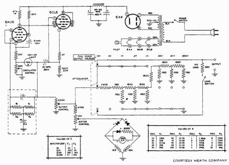
output increases the lamp current, the lamp temperature, and the lamp resistance. This reduces the amount of feedback applied to the 6AU6 cathode, and the output is thereby reduced. A balanced condition is thus obtained. The oscillator control is used to set the nominal output level.
