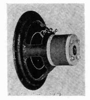
to have no resonance through a response range of 1 to 18,000 cps. With a five pound magnet and peak power of 20 watts, the loudspeaker employs one cone, sectioned, with a mechanical crossover that is said to avoid any break in tone. Cloth suspension is reported to allow cone movement of  $\frac{1}{2}$  in.
