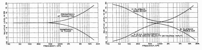
must provide a complementary amount of high-frequency droop and bass boost. Curve A in Fig. 2 shows the equalization used in recording, while Curves B and C show the equalization required in playback when a magnetic pickup is used.
