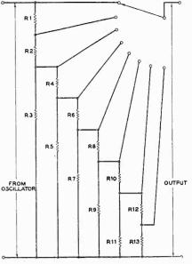
Fig. 7. The output attenuator section.
