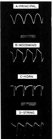
phase-shift amplifier which gives the signal a sharp, horn-like quality. The outputs of these two filters, together with the output of a filter fed by square waves, and a signal taken directly from the beat-frequency oscillator, are all connected to switch S<sub>3</sub>. The performer can select the timbre which he desires simply by setting this switch. Wave forms of the four timbres are shown in Figs. 5A through 5D.
