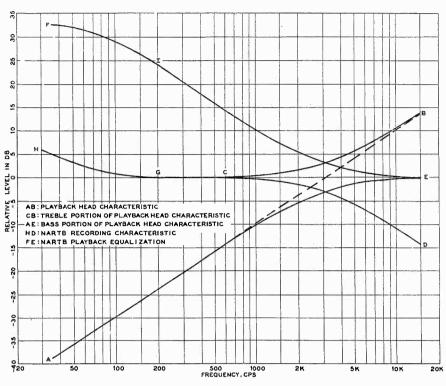
Fig. 8. How flat over-all response is achieved with optimum signal-to-noise ratio.
