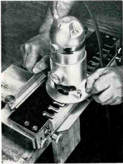
Fig. 3. Router and dovetail attachments.
