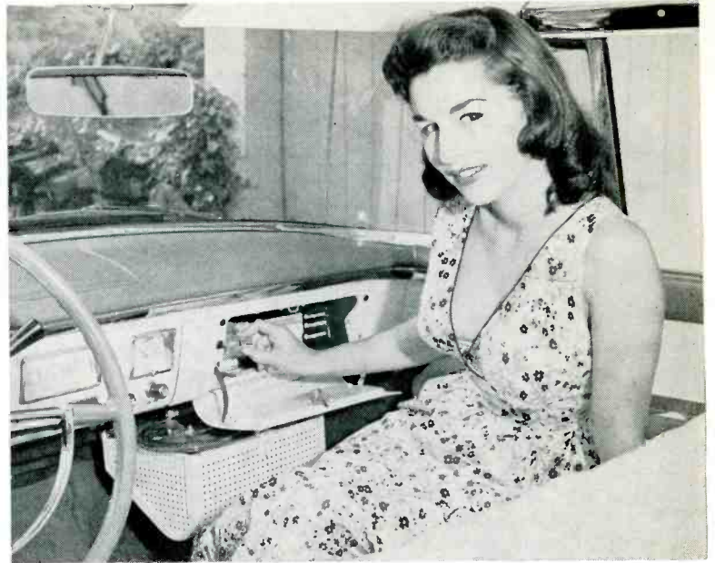
Tape playback preamplifier and several reels of tape fit comfortably in the glove compartment. Under the tape deck, visible below dash, is adequate foot room.
