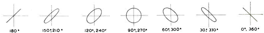
Fig. 5. Lissajous patterns for sine waves of same frequency and amplitude, with the phase relationships shown. These patterns can be used for rough estimates.
