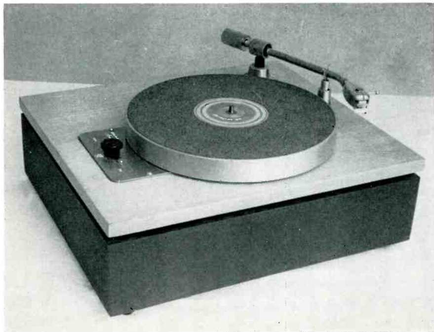
Fig. 1. Attractive homemade base for Rek-O-Kut L-37 turntable and 120 tone arm.
