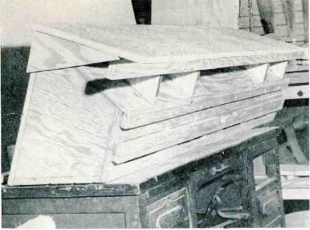
Resonating chamber and top panel of enclosure glued and screwed together. Strip of plywood was nailed to back edges of triangular braces, and scrap pieces of plywood were attached to each end, to serve as temporary guides in positioning top panel.
