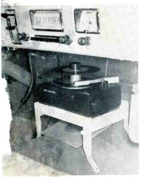
Player its ricely into the foam-rubber cushion, and plays through auto radio system. Power is obtained from inverter.
