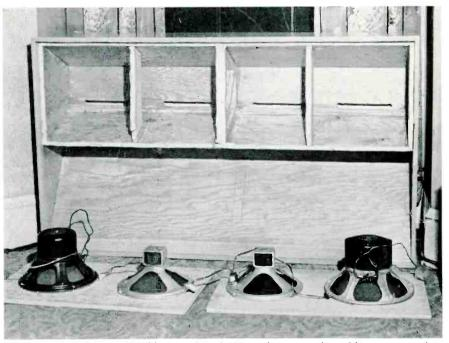
The upper and lower assemblies combined. Now the reason for adding top panel to the coffin is apparent: this very heavy unit simply rests in place while it is firmly attached to lower assembly. Two speaker mounting hoards simplify installation too.
