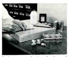
Laying out a chassis: colored pencil will not scratch aluminum surface and lines wash off with soap and water.
