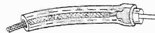
Plastic tubing makes phono pin-tip plug easier to handle, less likely to break.
