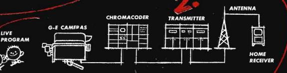
Excellent colorcasting results from either system, but Chromacoder, in fixed location, handles registration for all cameras in its system, and such adjustments are stable. See 3,5+7 for other advantages of fixed equipment.
