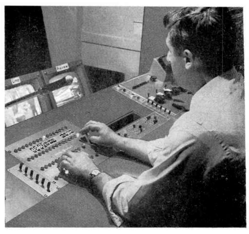
TS-1-A SYSTEM provides complete dissolve, fade, previewing, direct switching and sync mixing facilities for eight non-composite video inputs and two composite inputs. Provisions are also available for special effects.
