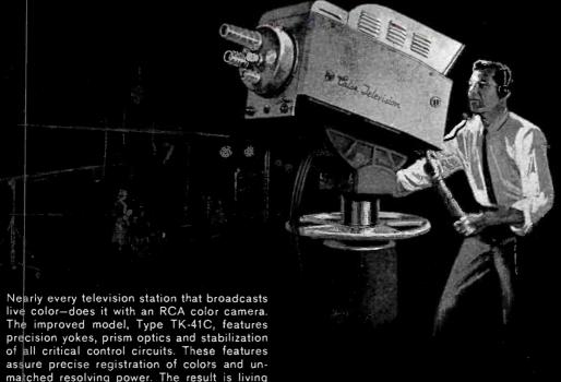
of all critical control circuits. These features assure precise registration of colors and unmarched resolving power. The result is living color performance.
