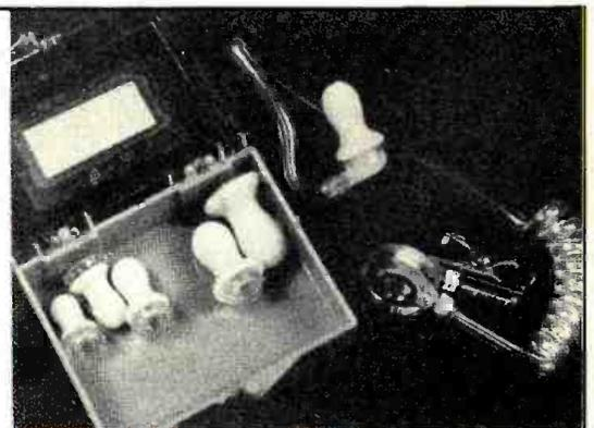
The On-Camera Audioclarifier is used mostly for talent. It comes with six different size ear tips or a custom ear piece. Both custom and tip models are also used for security and surveillance work.
