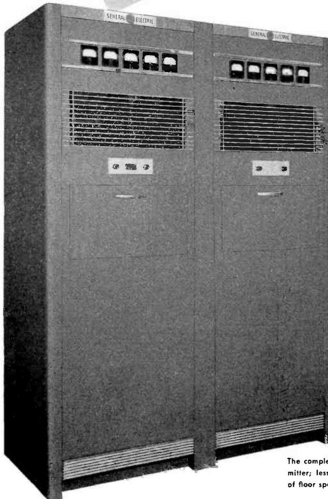
The complete G-E 1-kw FM transmitter; less than 10 square feet of floor space is required
