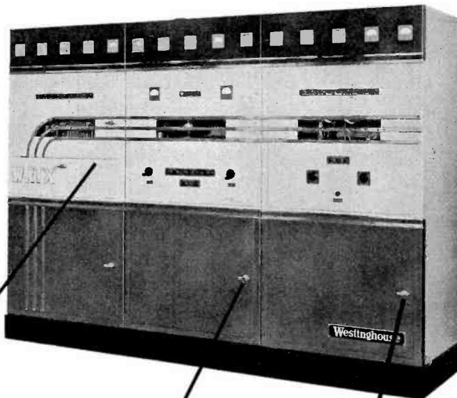
**MODULATOR CUBICLE**—Lower door opens to make it easy to check relay operation.
