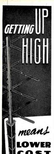
Getting that F-M Antenna up high not only means more efficient area coverage-but it also means lower costs. Doubling the height of the antenna above ground is equivalent to squaring the transmitter power. Thus, a 250 watt transmitters with a 200 foot tower would equal a 1000 watt transmitter with a 100 foot tower. That is real economy—both in initial transmitter cost and in power.
