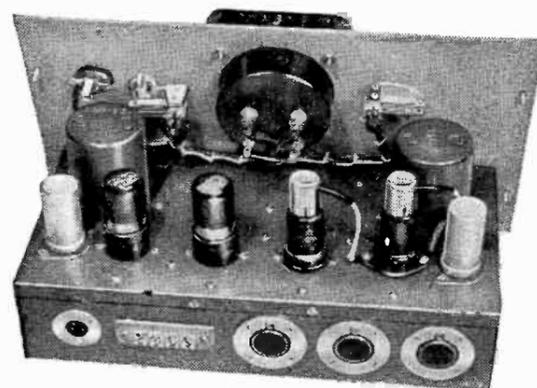
Entire chassis of both amplifiers and power supply instantly slides out of cabinets by merely turning four air lock screws on front panels. Provides complete accessibility to all components and wiring for emergency servicing. Supplied with either Cannon or Hubbell plugs.
