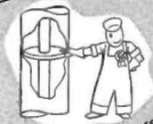
Inner conductor is securely anchored inside each section for fixed electrical characteristics.
