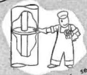
Inner conductor is securely anchored inside each section for fixed electrical characteristics.
