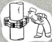
Differential expansion is automatically compensated at 20 foot intervals in SEAL-O-FLANGE Lines.
