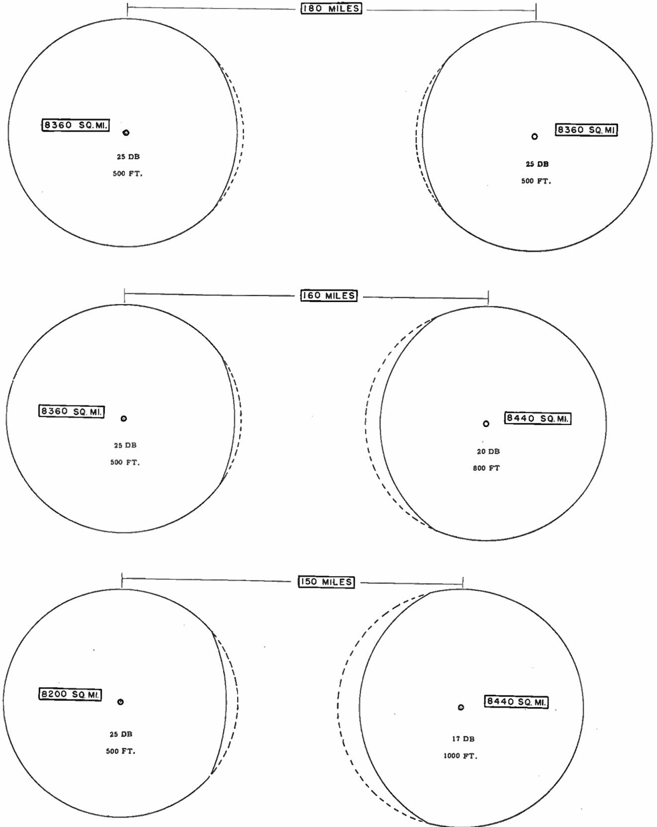
NOTE: Diagrams above portray television station interference free "B" service areas for channels 7-13 (solid lines) based on standard interference and separations of 150, 160 and 180 miles, including offset carrier operation. Essentially equivalent service areas are obtained by varying the parameters - antenna height, power and station separation. Dotted lines show potential coverage without co-channel interference.
