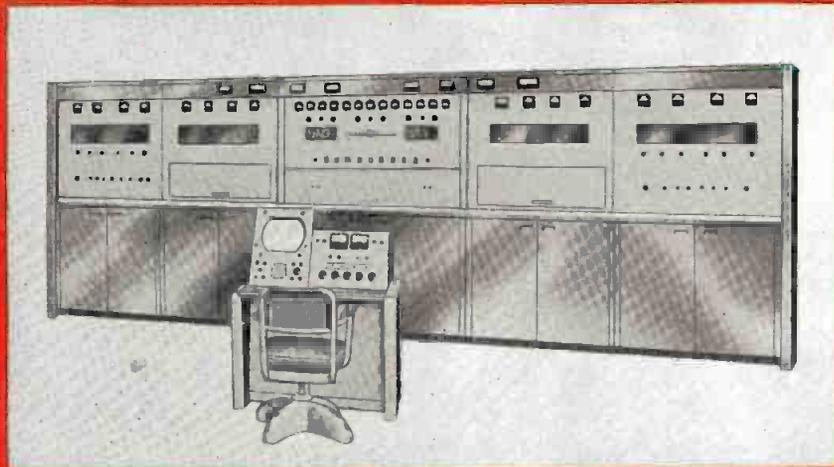
**World's Most Powerful UHF Television Transmitter.** This 12 kw unit offers a unique frequency control system. One crystal oscillator controls both the visual and the aural carriers, locking them together with a fixed separation of 4.5 mc. A number of broadcasters have already placed orders for this UHF transmitter.
