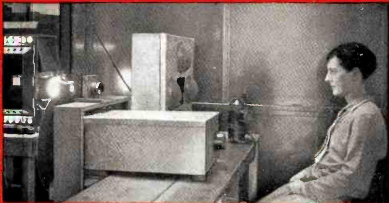
**First Television "Camera."** As light from electric arc at left is projected through 48 holes of revolving disc, the flashes are picked up by 4 electric eyes protruding from wooden frame on table. The impulses are then broadcast much the same as any radio message.
